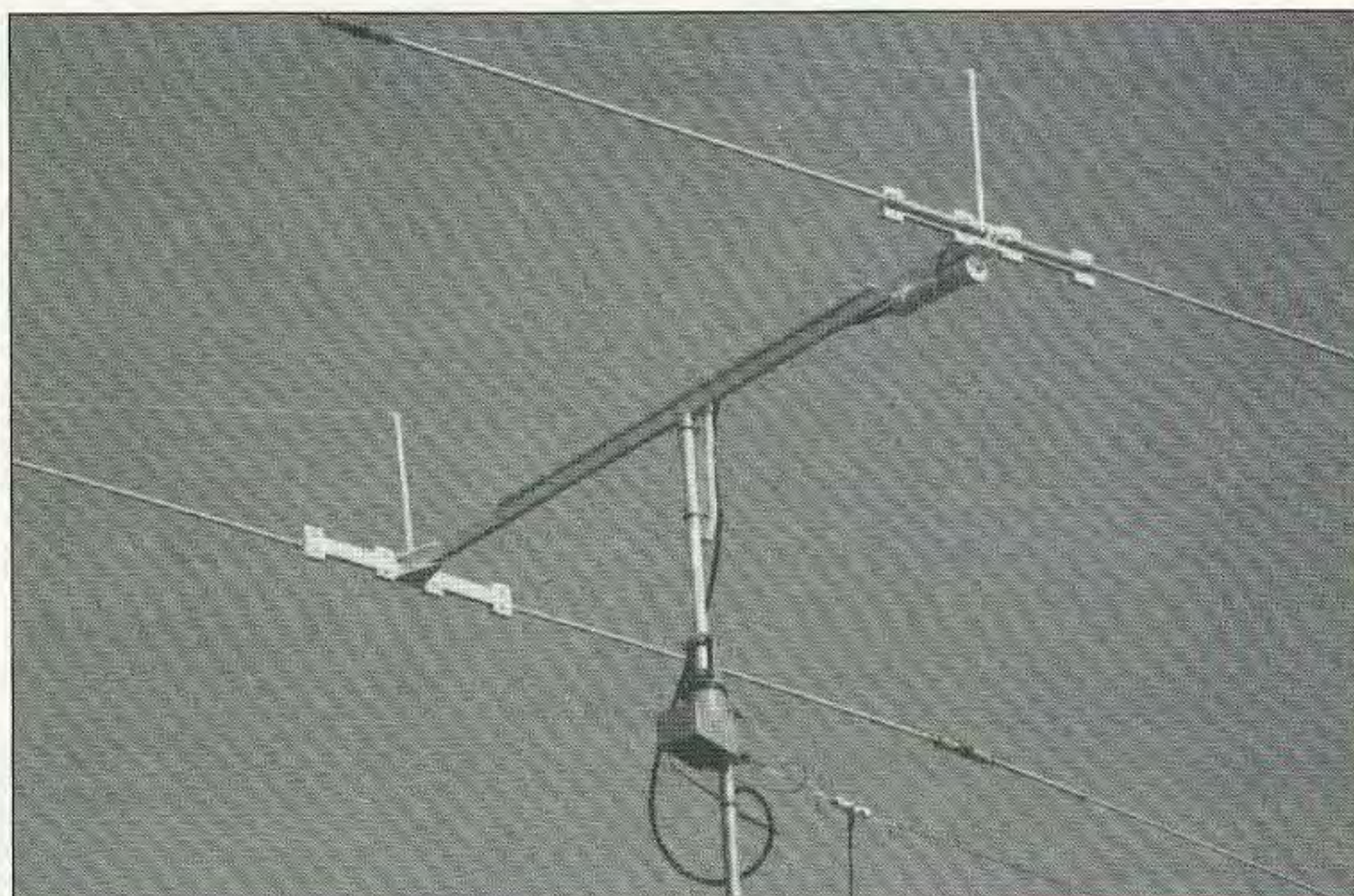
Photo A. The completed 20 meter mono-bander.
