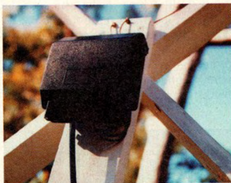
Above: A close-up of the completed antenna. The waterproof enclosure is available from Oatley Electronics and is used here to house the PCB that mounts at the antenna.
