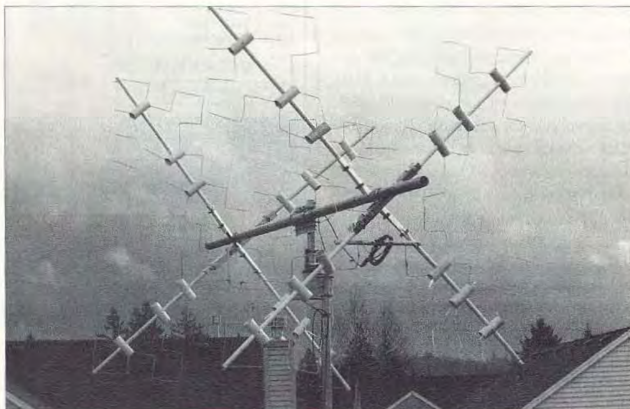
Photo A. The 2-element FQY mounted at the author's home. The element spacing here is 6.5 feet.
