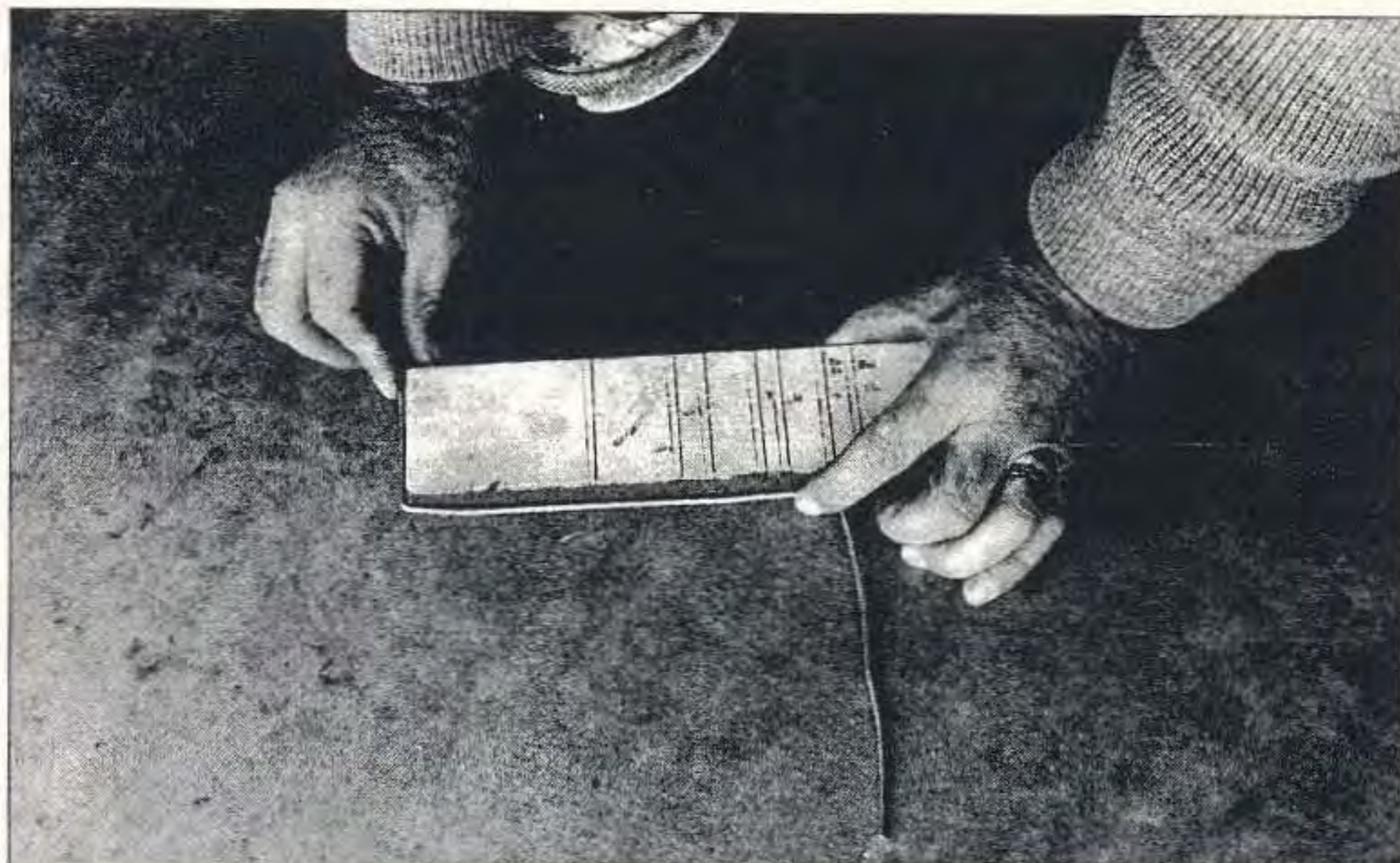
Photo B. Bending the wire around a wooden block. The block is marked for the different length bends.
