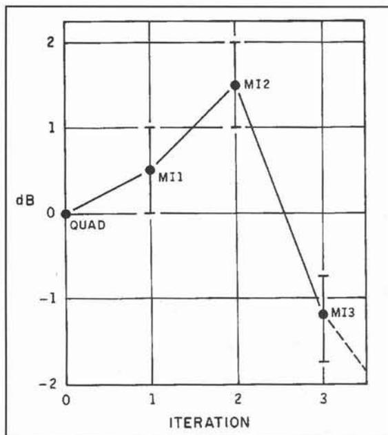
Figure 12. Strange gain changes with iteration for lowest resonance of the MI fractal antennas. This may be a diffraction phenomenon and is not due to losses from inefficiency.
