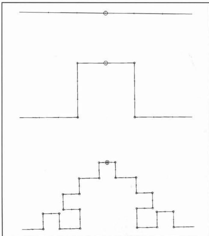
Figure 7. Minkowski (box) fractal for iterations 0, 1, and 2.
