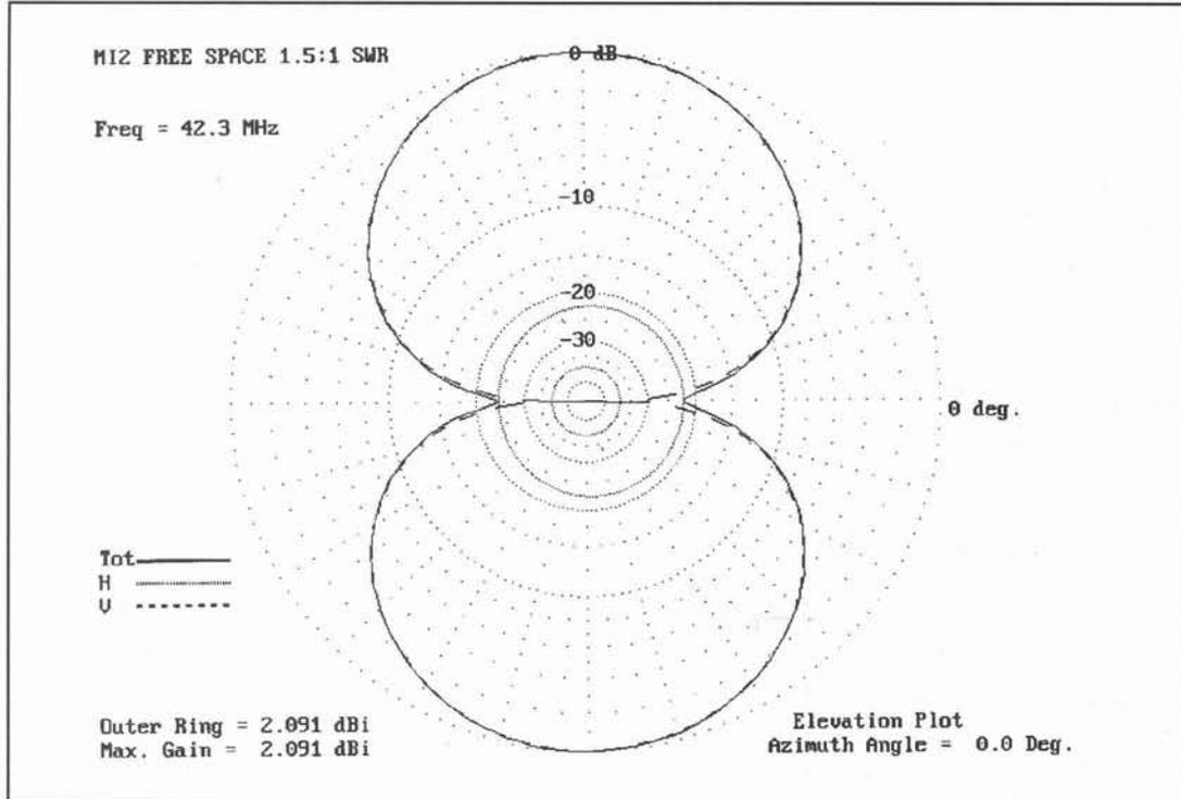
Figure 11. Free-space pattern for MI2 from ELNEC. This pattern is very similar to that of a quad, except with 2 dB less front to side and 1 dB less forward gain; a little lower than measurements show.
