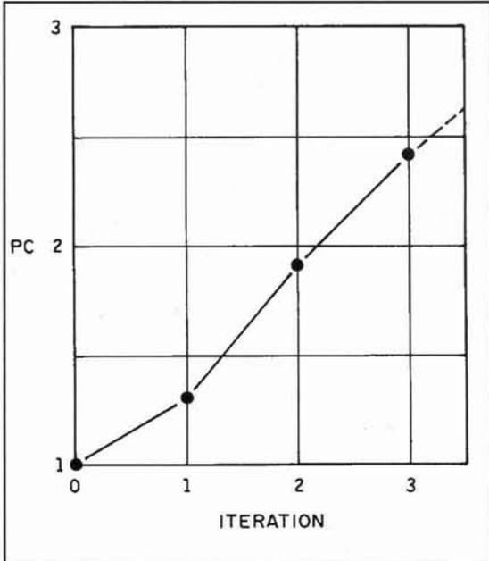
**Figure 13.** PC has not topped out with iteration 3 of the MI fractal antennas. There's further shrinkage to be had!
