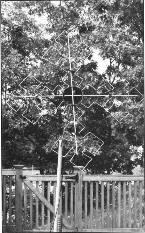
Photo B. A picture of MI2 for 6 meters—about 30 inches on a side. Ready for an efficiency measurement. Note easy support to spreaders at many points.
