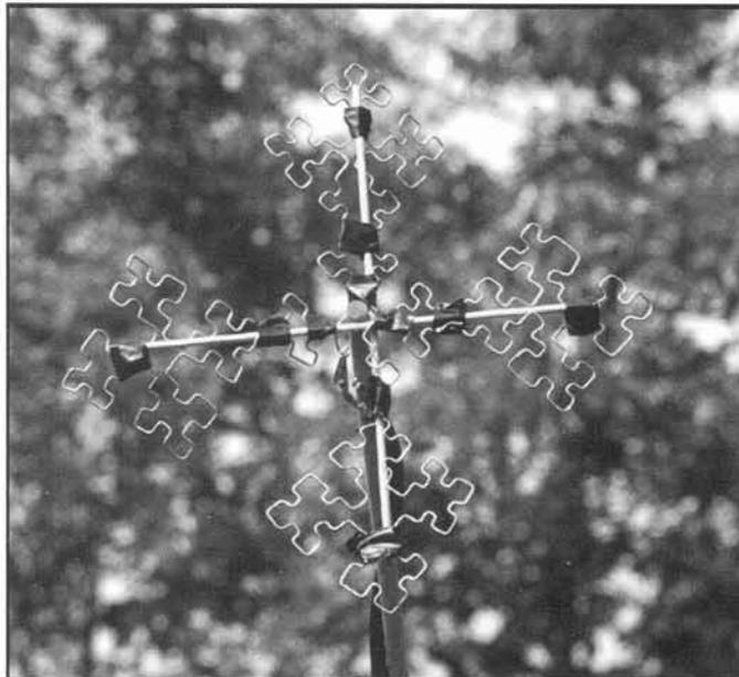
Photo A. A picture of MI3 for 2 meters—about 8 inches on a side. Now to stick it out the window!
