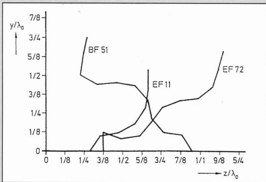
Figure 16. Adapted from Landstorfer and Sacher, 1985. These bent lines represent optimum shapes for a vertical element. Who needs a straight line?
