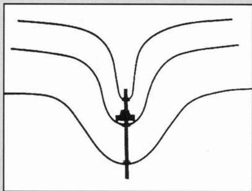
Figure 15. Adapted from Landstorfer and Sacher, 1985. Oddly shaped Yagi, but it has 3 dB more than a regular one.
