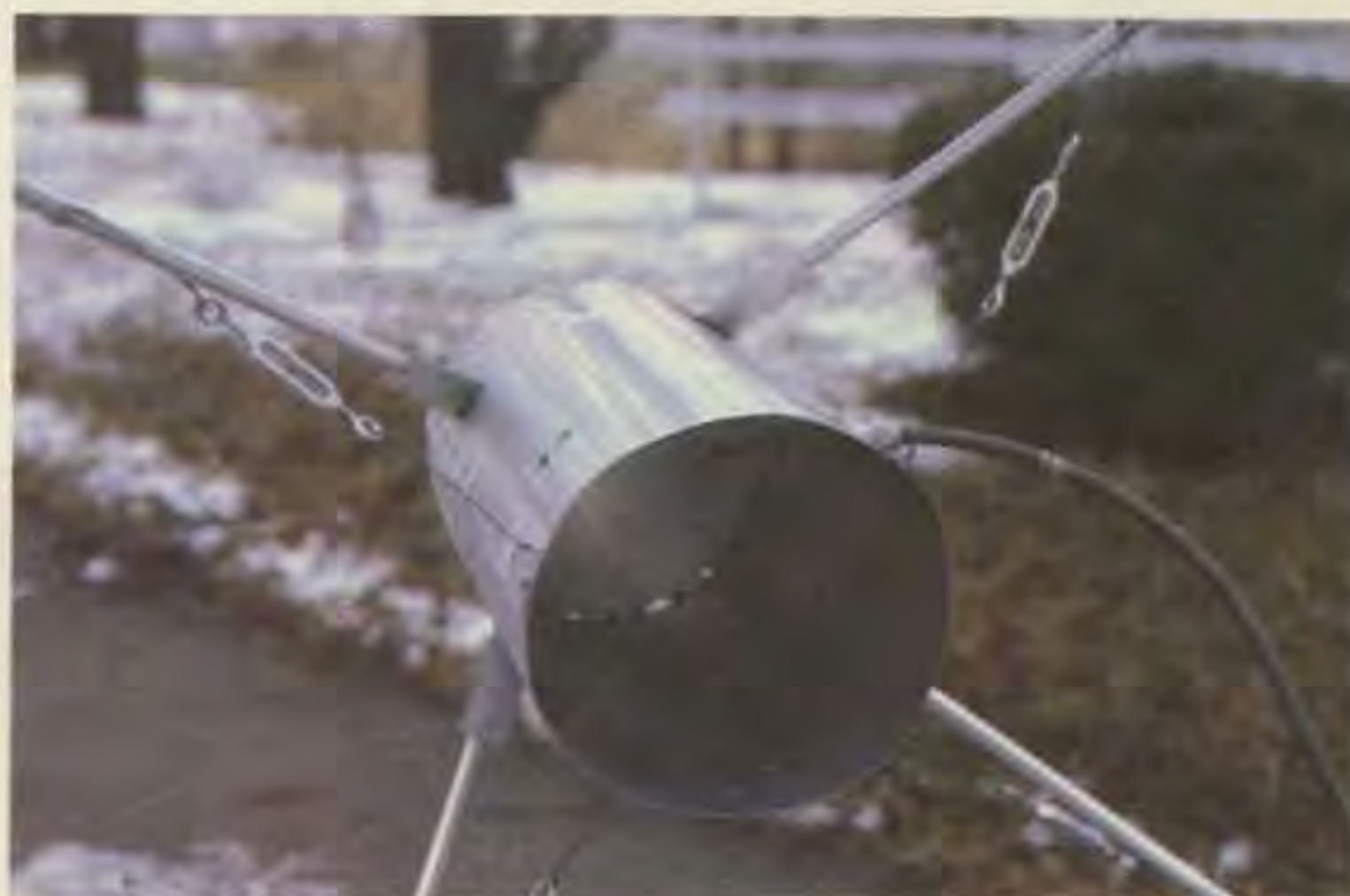
Photo B. A feedhorn can be easily constructed. The pickup is a simple, monopole element.
