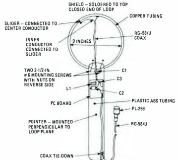
FIG 1—A LOOP ANTENNA can easily be built using some copper tubing, some plastic tubing for the mast, and a few components. It can help you locate the source of troublesome TVI, or find the position of someone who is in need of help.
