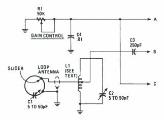
FIG. 3—THE BASIC circuit to tune the loop antenna. Coil L1 consists of 25 turns of #24 magnet wire, tapped at 6 turns from the low end, on a ¼-inch form.
