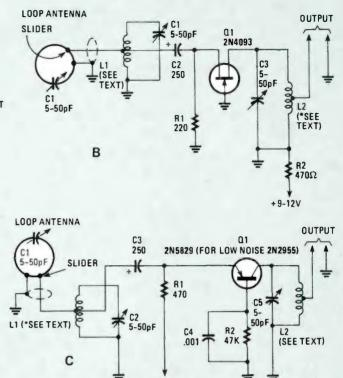
dummy-load for 5-watt CB rigs. With the two units some distance apart, adjust C1, C2, and the slider on the loop with an alignment tool for a peak indication on your S-meter. The adjustments will interact, and if one or more adjustments won't peak the S-meter. try adding a 10- to 20-pF capacitor across C1.
