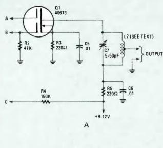
FIG. 4—THREE PRE-AMP CIRCUITS you can put together tonight! If a preamp, is needed any one of those three circuits will serve. The circuit shown in *A* offers the advantage of an adjustable gain control. Liberal substitutions may be made as the values are not critical.
