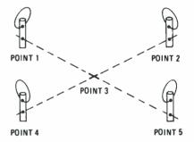
FIG. 2---TO PINPOINT a location, at least two readings should be taken. The point where the lines determined by those readings intersect is the general location of the transmitter. The more readings that are taken, the more precisely a location can be found.
