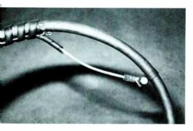
END OF COAX BRAID is soldered to the top-center of the copper loop and the center conductor of the cable is connected to the slider that is made from a piece of copper.
