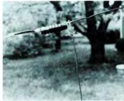
FIG. 3—Clipped on frequency-shift segments (2 required) lowers antenna resonance to CW frequencies.
