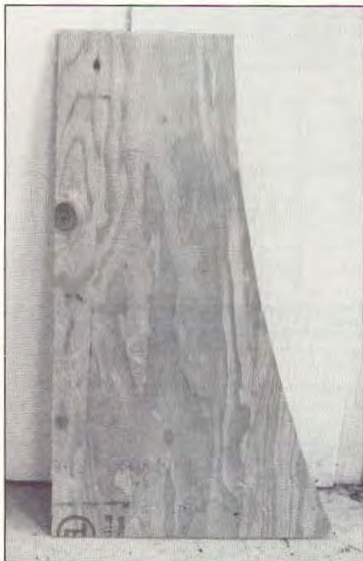
Photo A. Plywood bending fixture.
