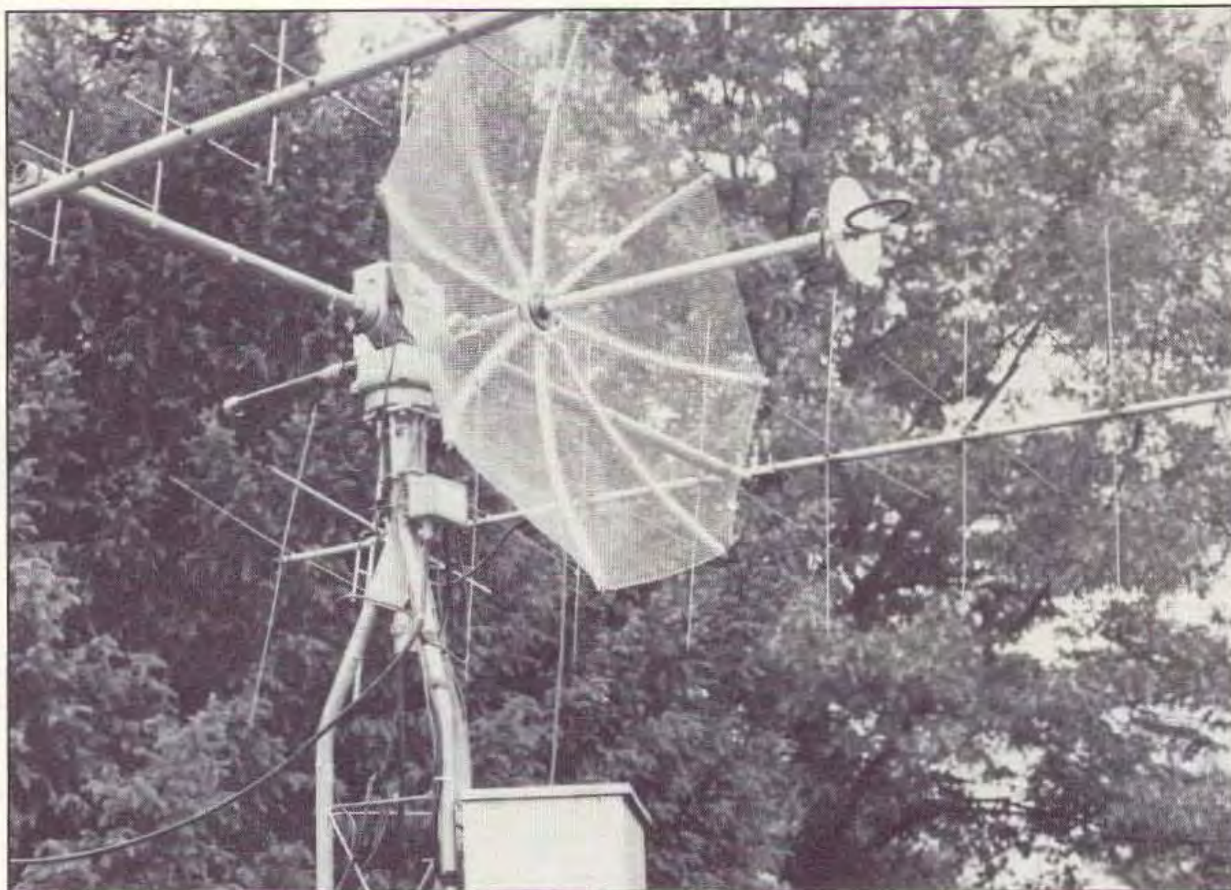
Photo C. Completed dish in place on the rotating bar.
