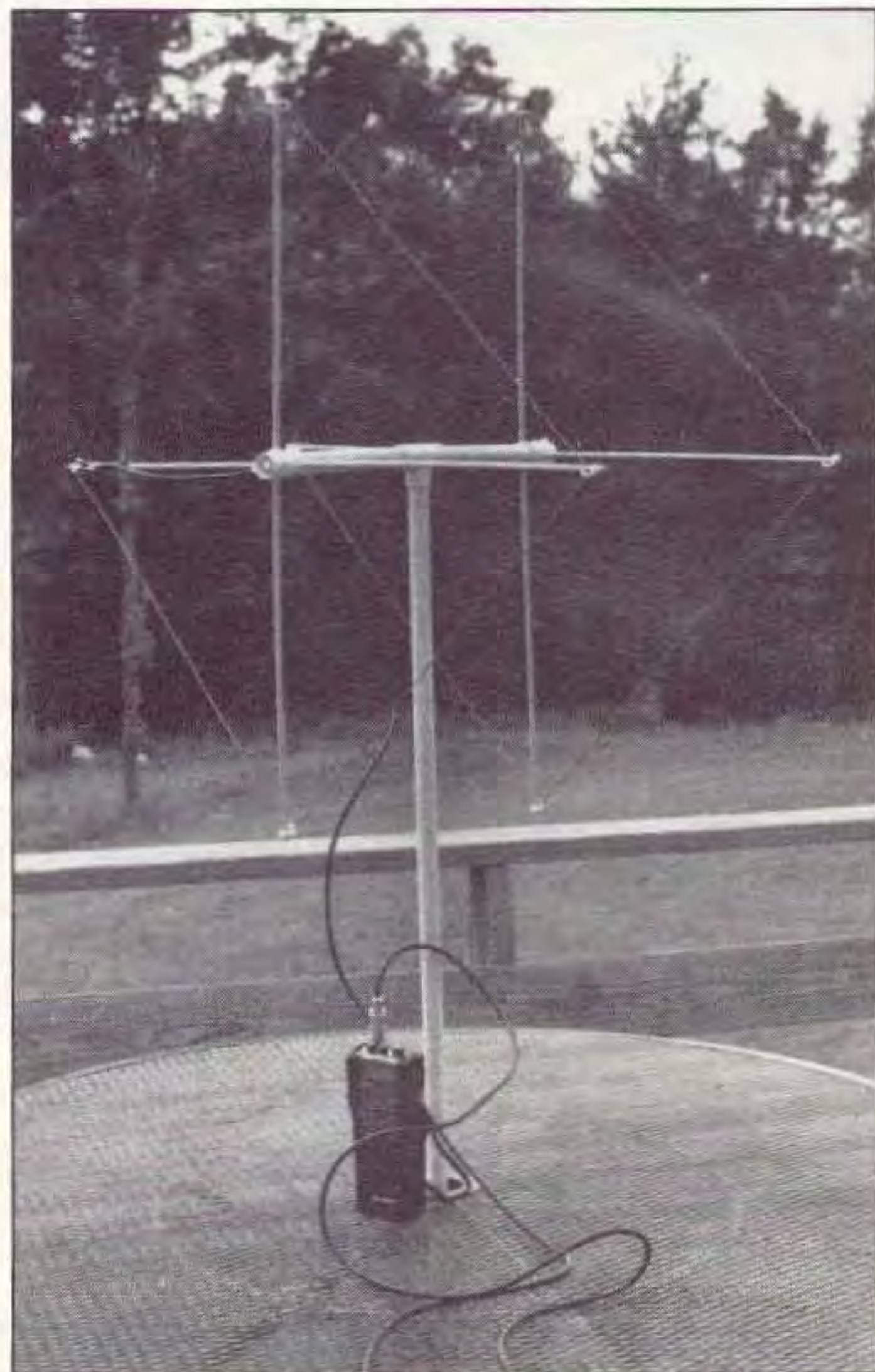
Photo A. The quad shown fully erected. Additional pieces of PVC piping can be added to the mast if more height is needed.
