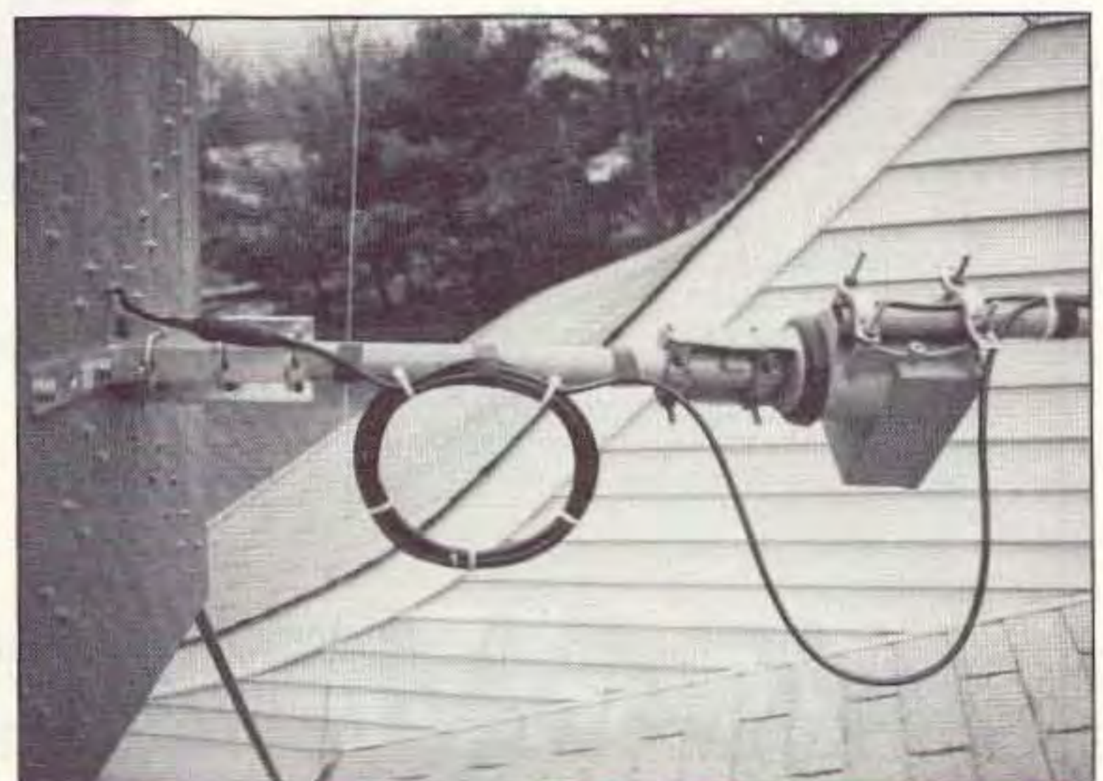
Photo F. Side view of current balun (RF choke) on antenna.
