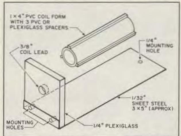
Figure 2. Matching coil platform.
