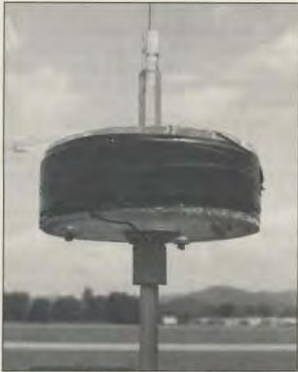
Photo B. Close-up view of the loading coil.
