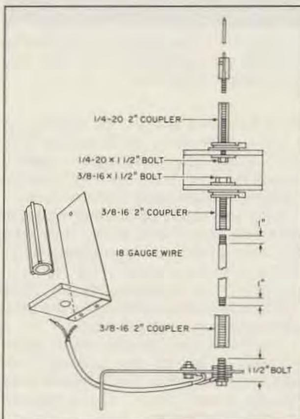
Figure 3. Overview of the mobile antenna.
