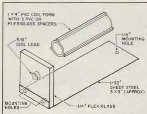
Figure 2. Matching coil platform.
