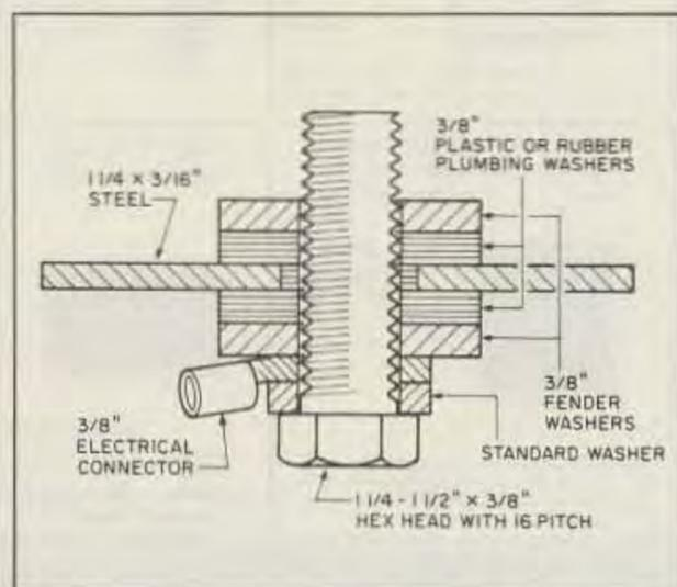
Figure 1. Antenna bracket.
