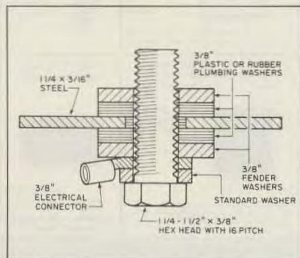
Figure 1. Antenna bracket.
