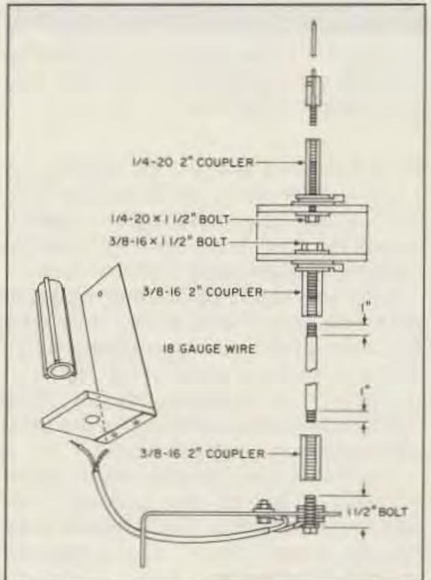
Figure 3. Overview of the mobile antenna.
