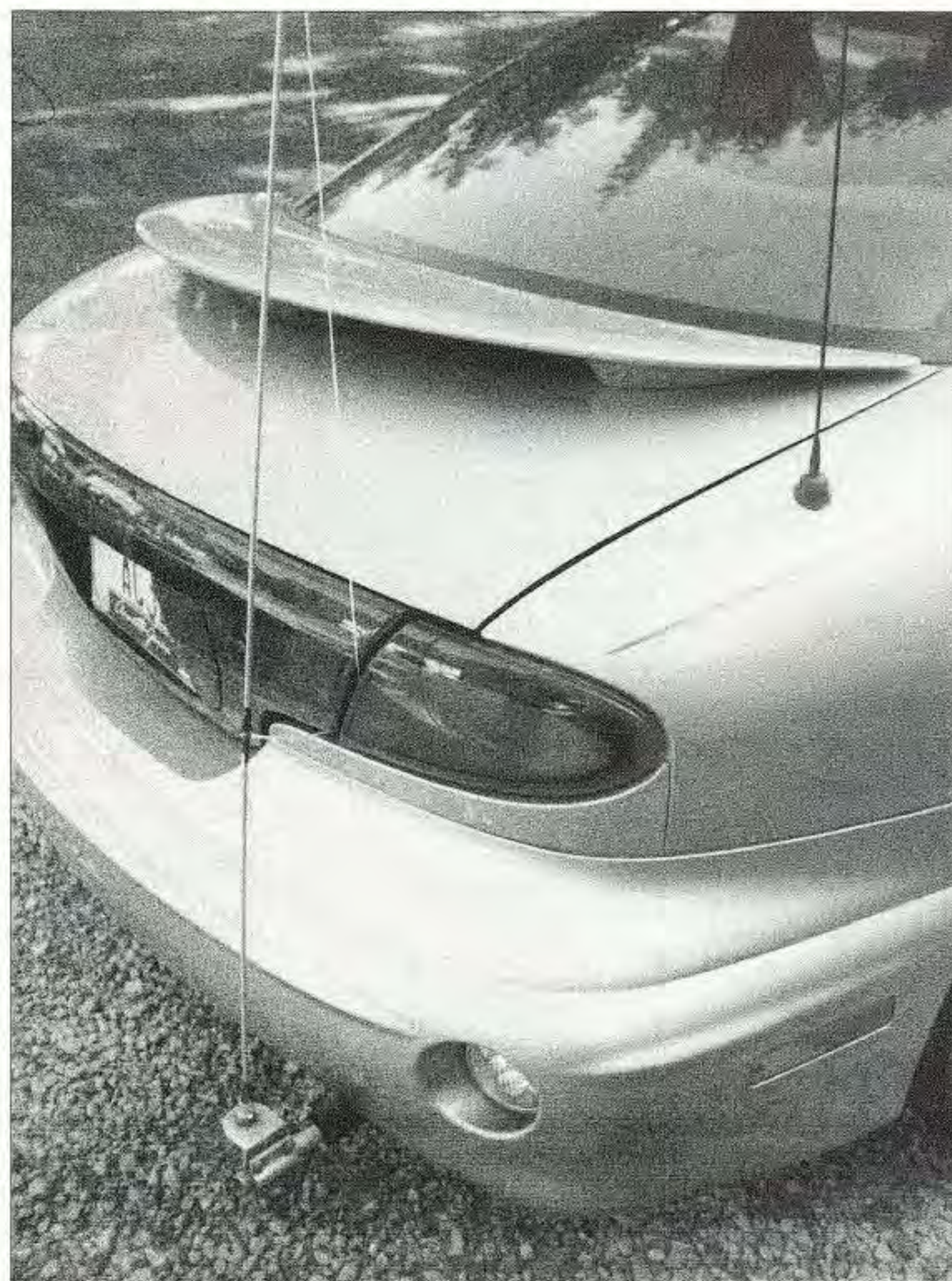
Photo A. Stabilizer tie-up.
