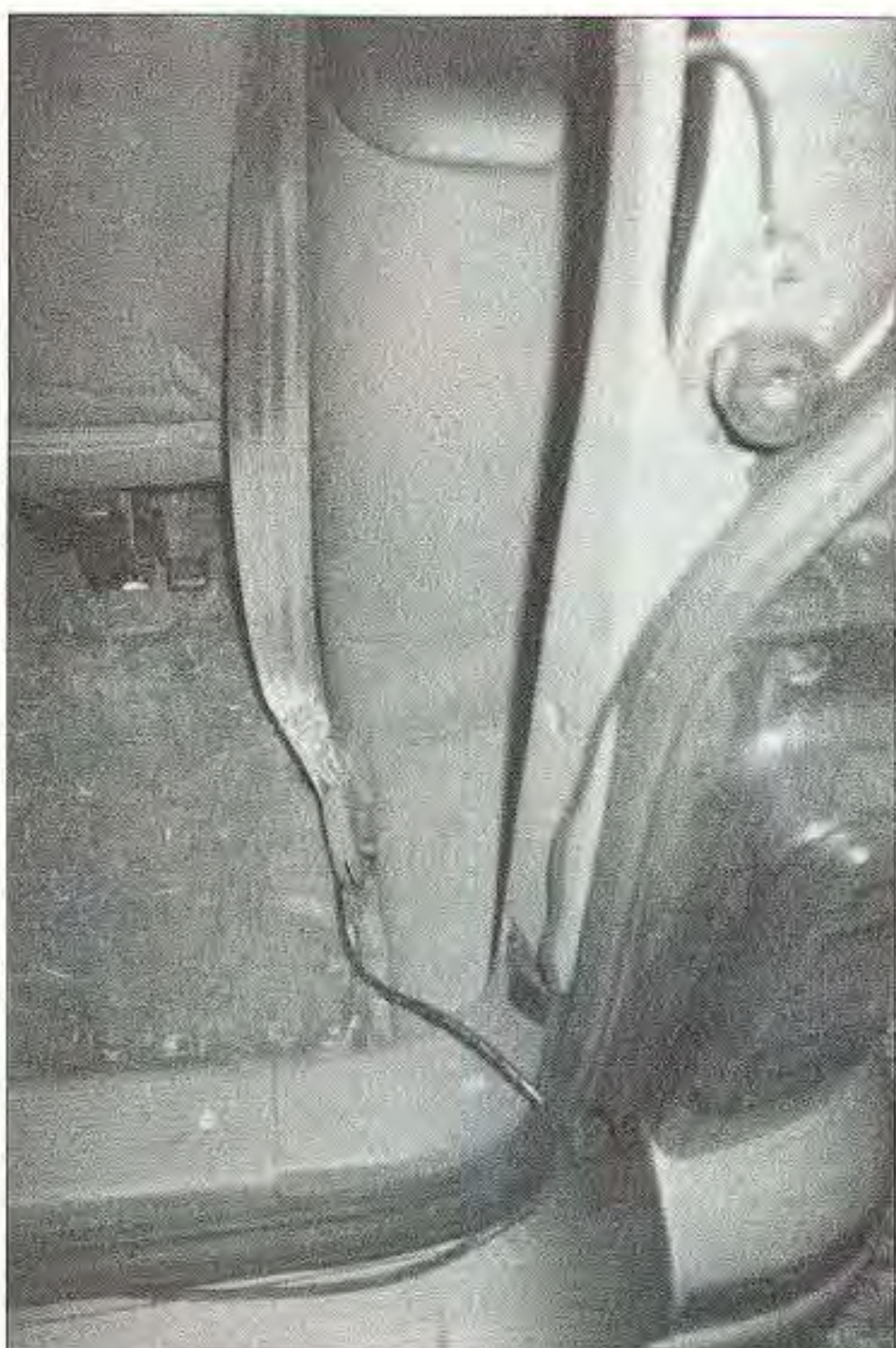
Photo C. Slip the cable into the trunk through the water seal if there are no water holes that you can use.
