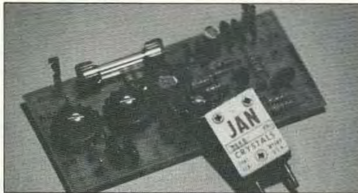
Photo A. The SW-1 QRP transmitter.
