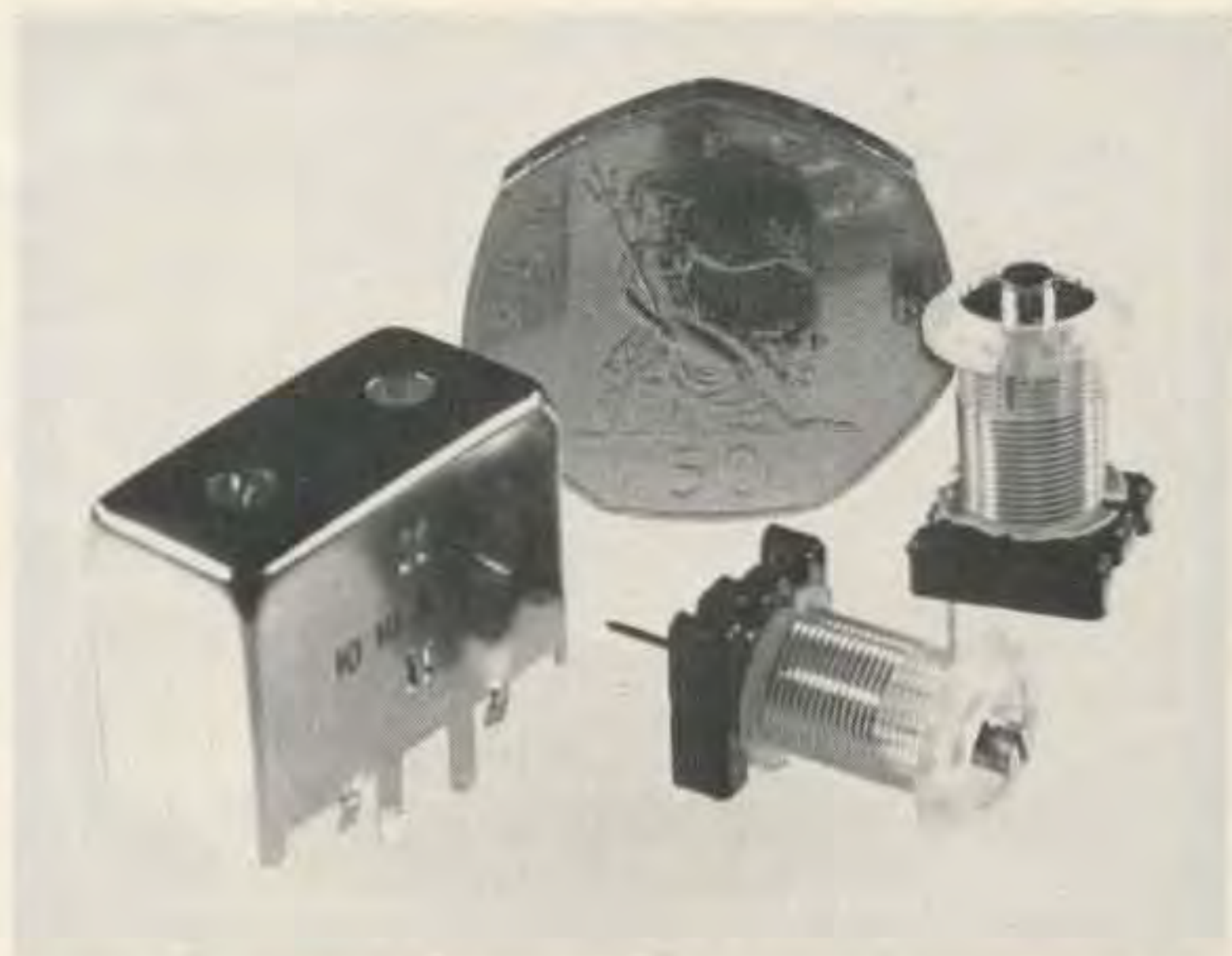
Photo B. An exploded view of the 2-pole version of the helical filter.
