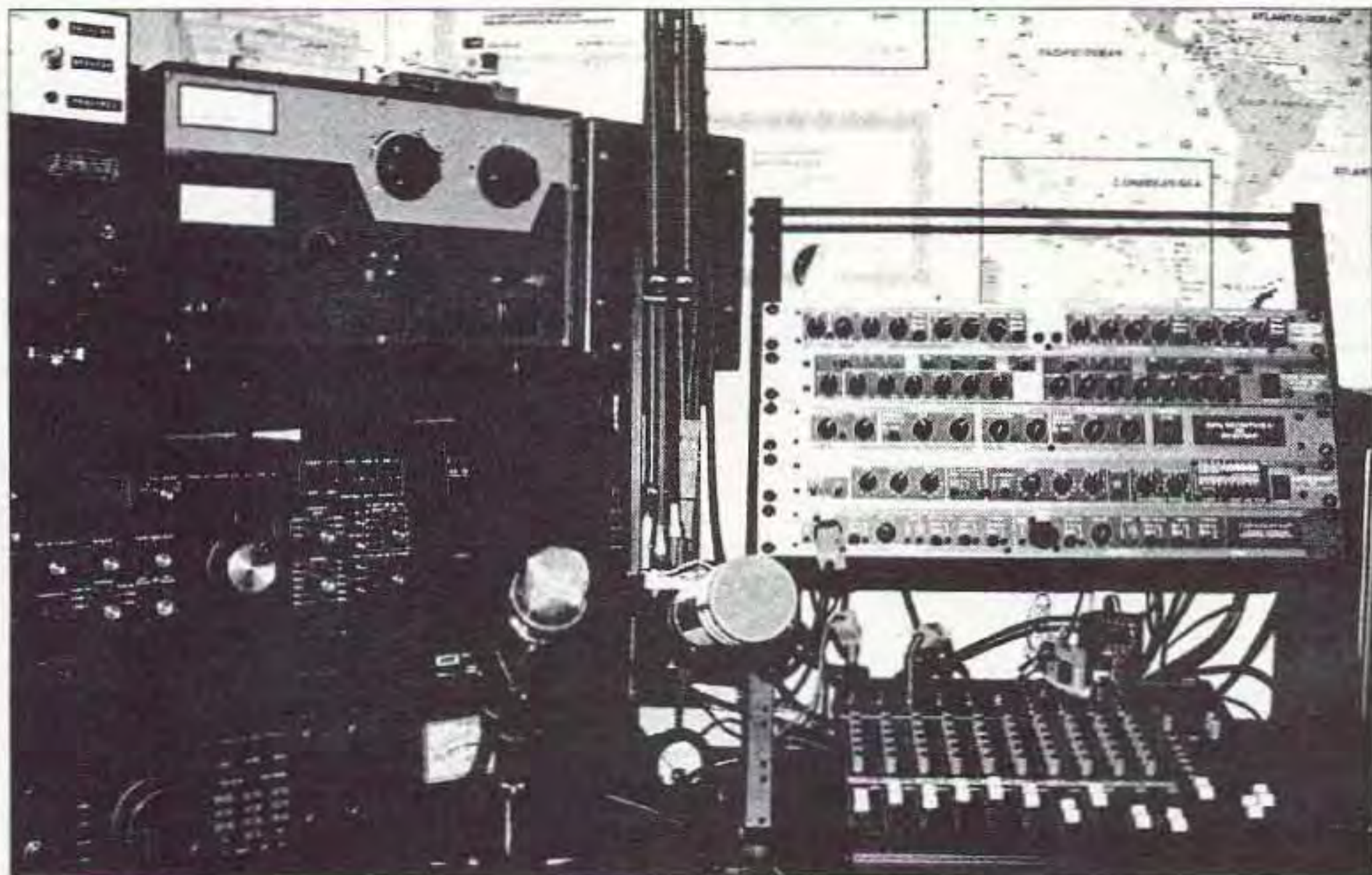
Photo D. John Basilotto W5GI gives us a peek at his secret ingredients for cooking up a super sounding signal. A Heil GoldLine mike connects to Aphex audio equipment consisting of a four-band parametric equalizer, an aural exciter, a "big bottom" booster, a compressor, a limiter, a reverb, and a mixer. Audio is then routed to his Icom 761 and Drake L4B amp. Whew!
