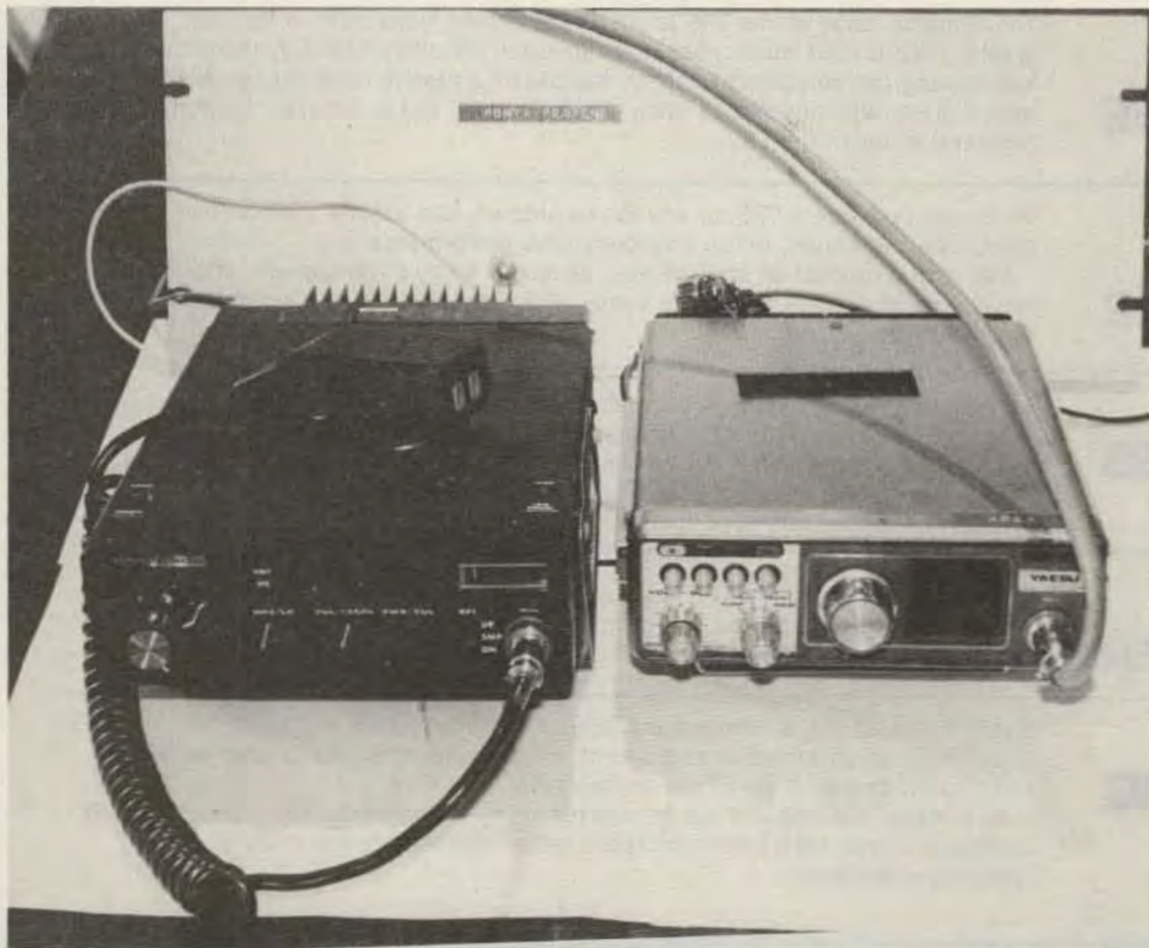
Photo A. Field Porta-Peater hookup with FT-227 and Tempo VHF-1. This Porta-Peater is housed in a minibox on a 19" rack panel (original prototype).
