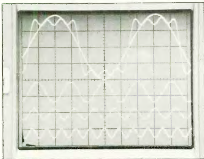
Fig. 2. Making of a square wave involves addition of fundamental frequency with odd harmonics. Third, fifth and seventh harmonics shown here are on the way toward making a square wave.
