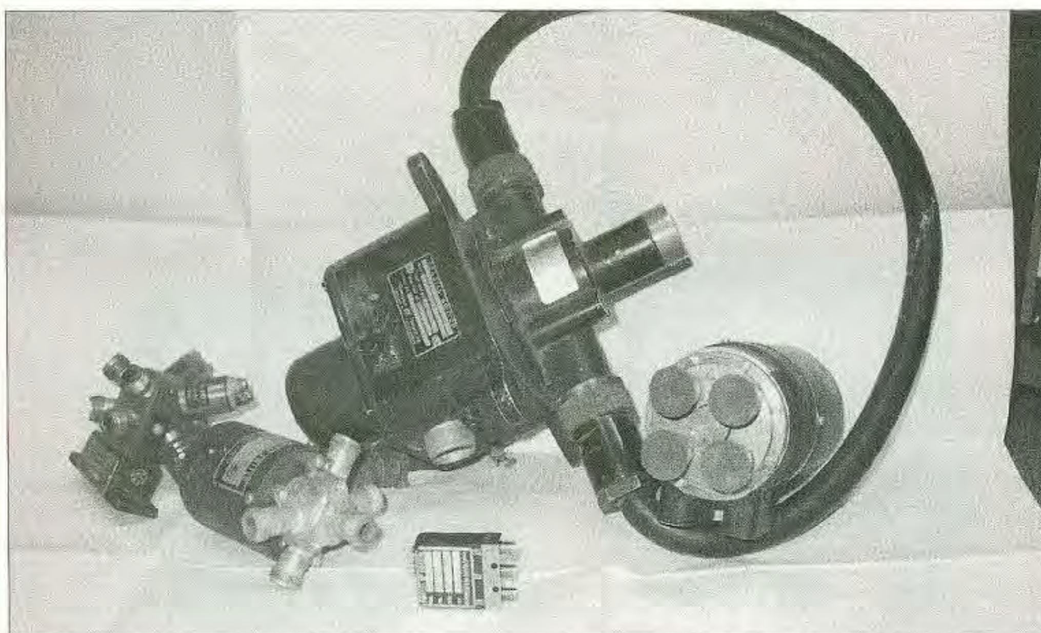
Photo E. Now, just when you think you have seen everything, here is a coaxial relay, with connectors, that weighs in at seven pounds. A short section of coax cable is attached with connectors on each end, contributing a half pound. Consider this relay in the multi-multi-kilowatt level. Shown with smaller "N"- and SMA-type relays for size comparison; miniature SMA shown center front is 1-inch square.
