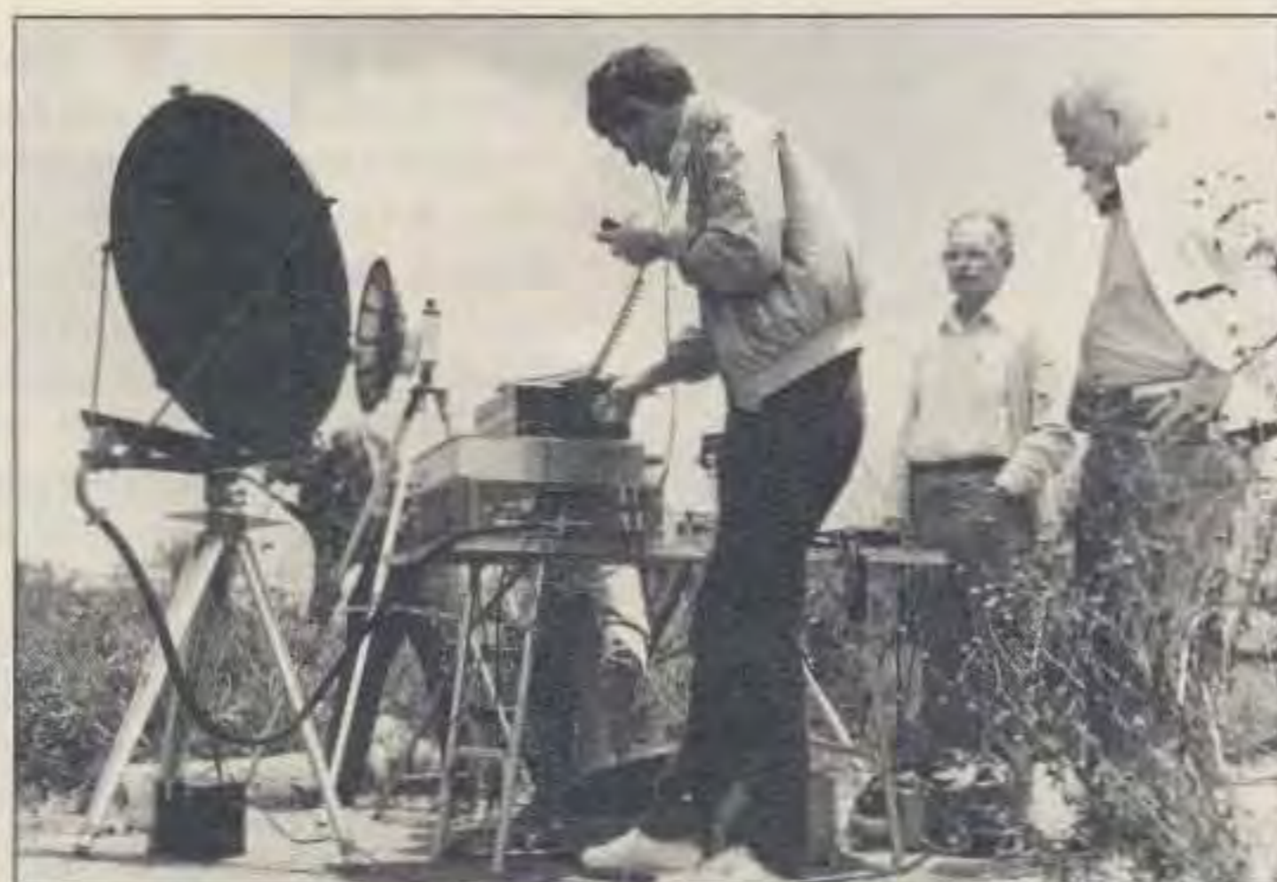
Kelly N6IZW operating the W6OYJ Polaplexer and 10 GHz SSB transceiver from the top of Mt. Soledad in California, while several other members of the San Diego Microwave Group look on. The transceiver drives a 10W traveling wave tube (TWT) amplifier. They made a contact over a 174 mile path, to a receiving system on Mt. Pinos. [Photo by author.]
