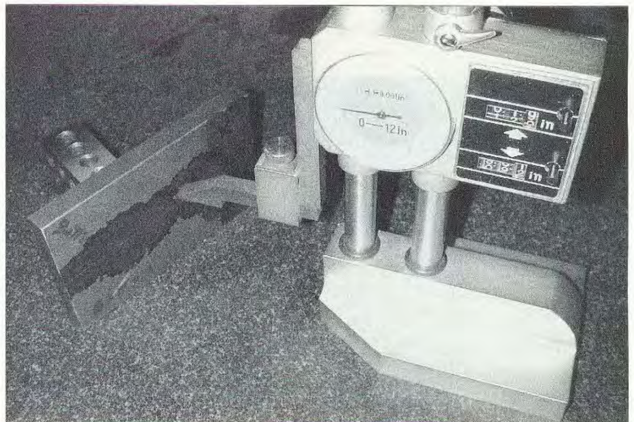
Photo G. Marking the base plate using a height gauge.
