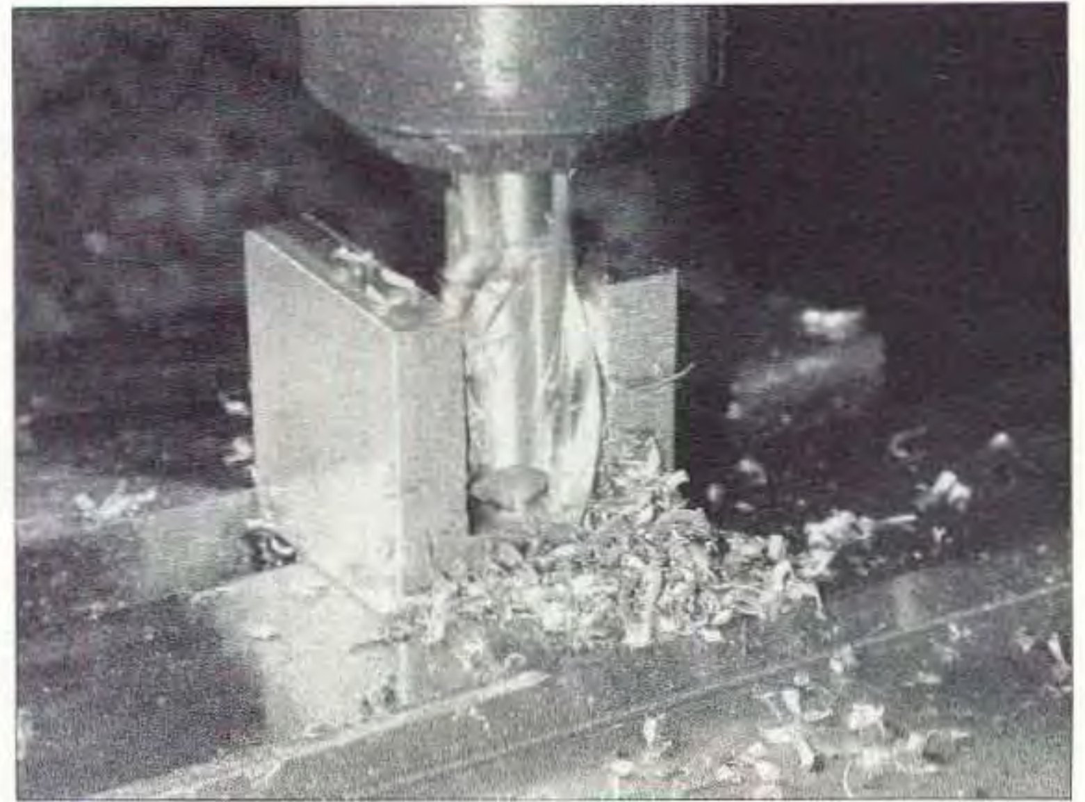
Photo B. Milling the bearing block.
