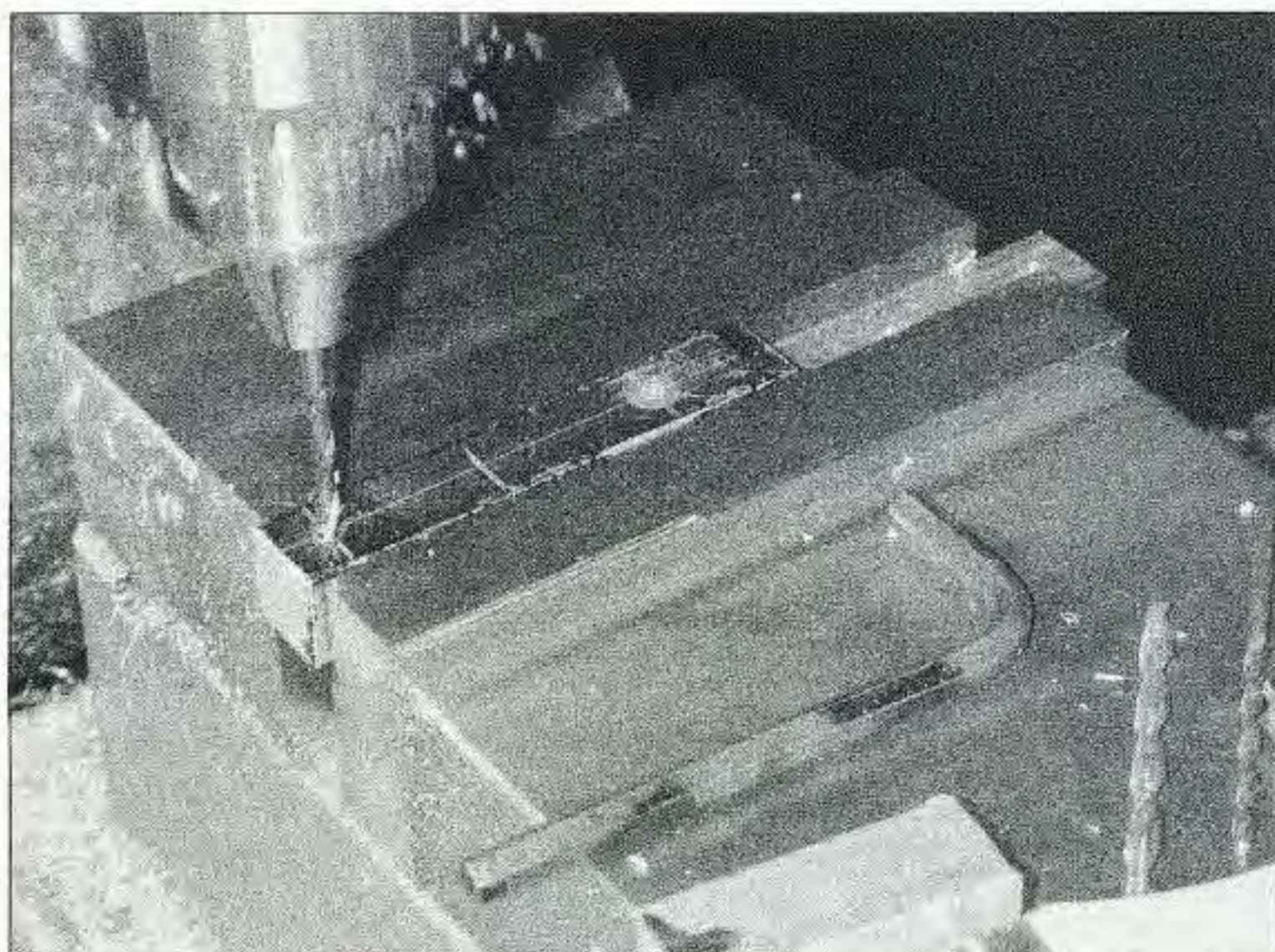
Photo E. Drilling the armature.
