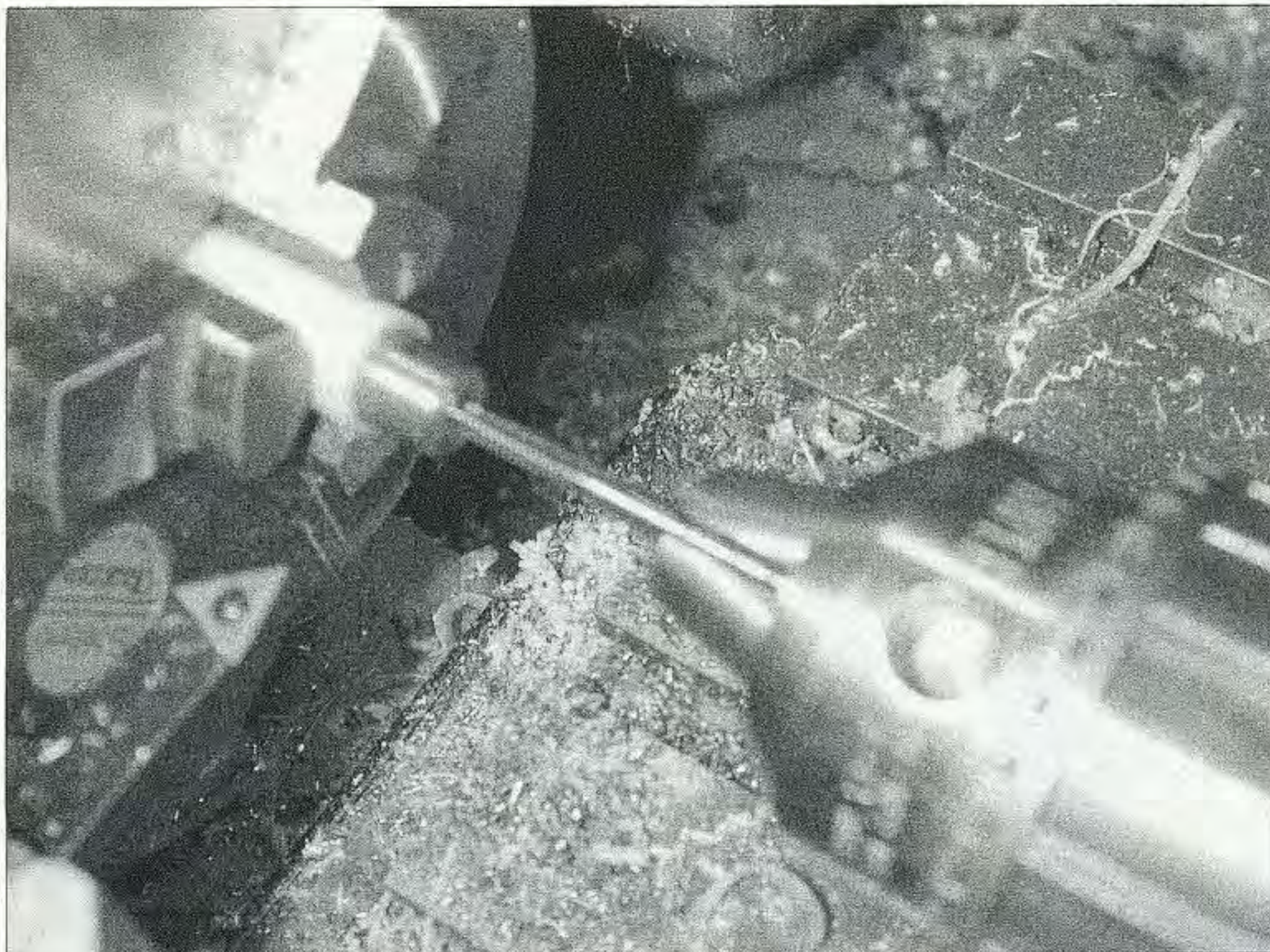
Photo H. Use a plastic bushing to prevent marking the connection posts while drilling and tapping.
