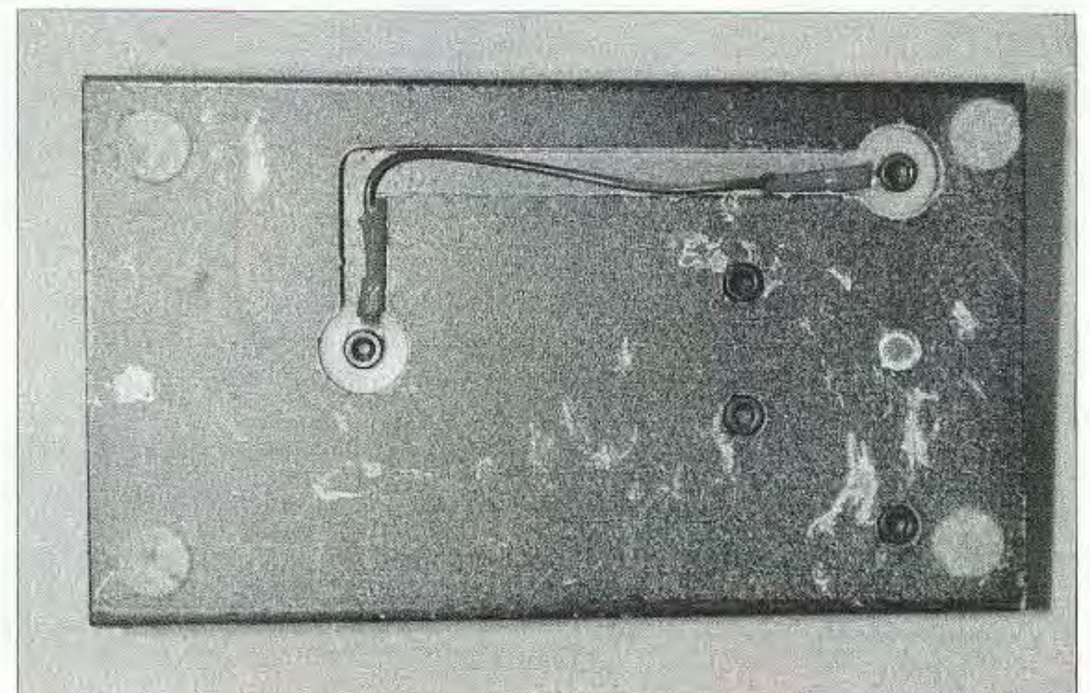
Photo L. Route the connecting wire through a milled channel.
