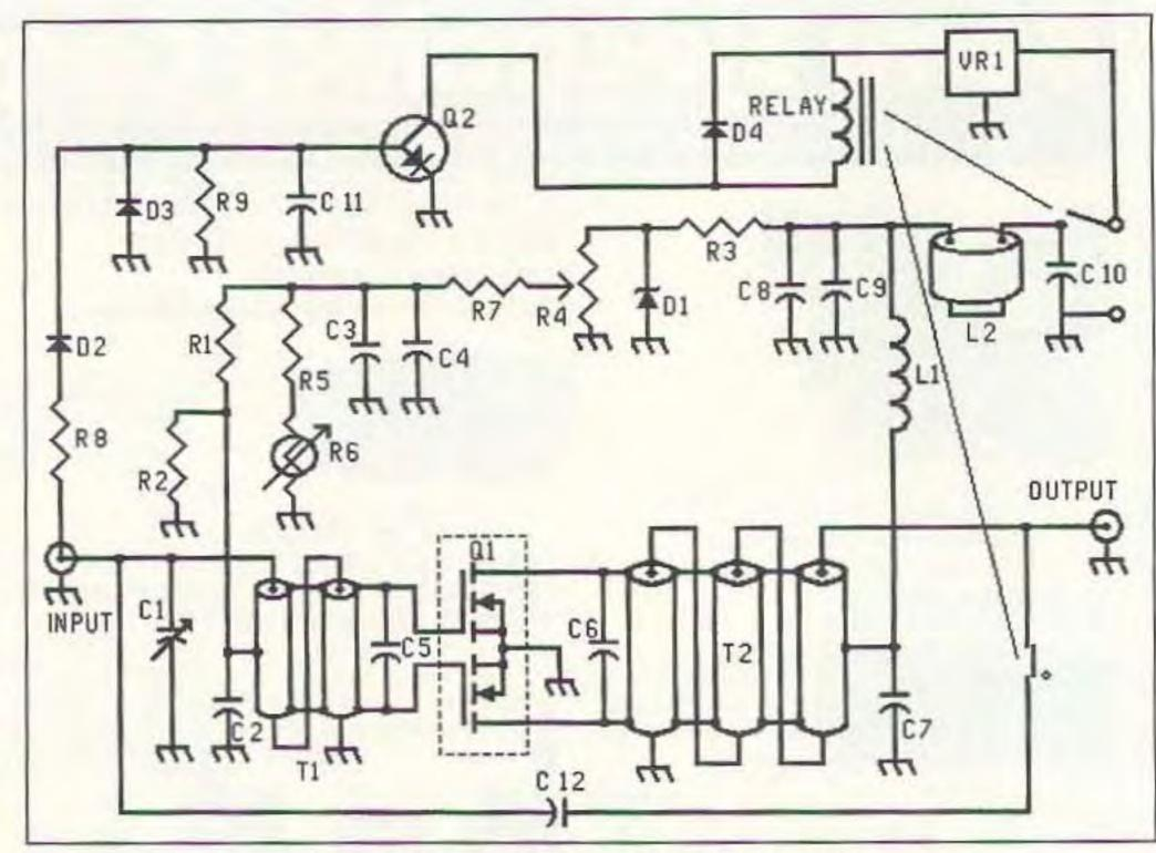
Figure 1. Schematic for the MRF175GV amplifier.
