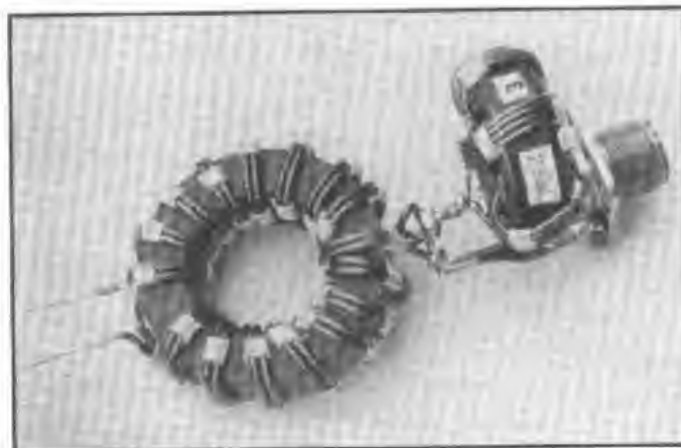
Figure 2 - A view of the compound-balun W2FMI-2.25:1-HB112.5 transformer.
