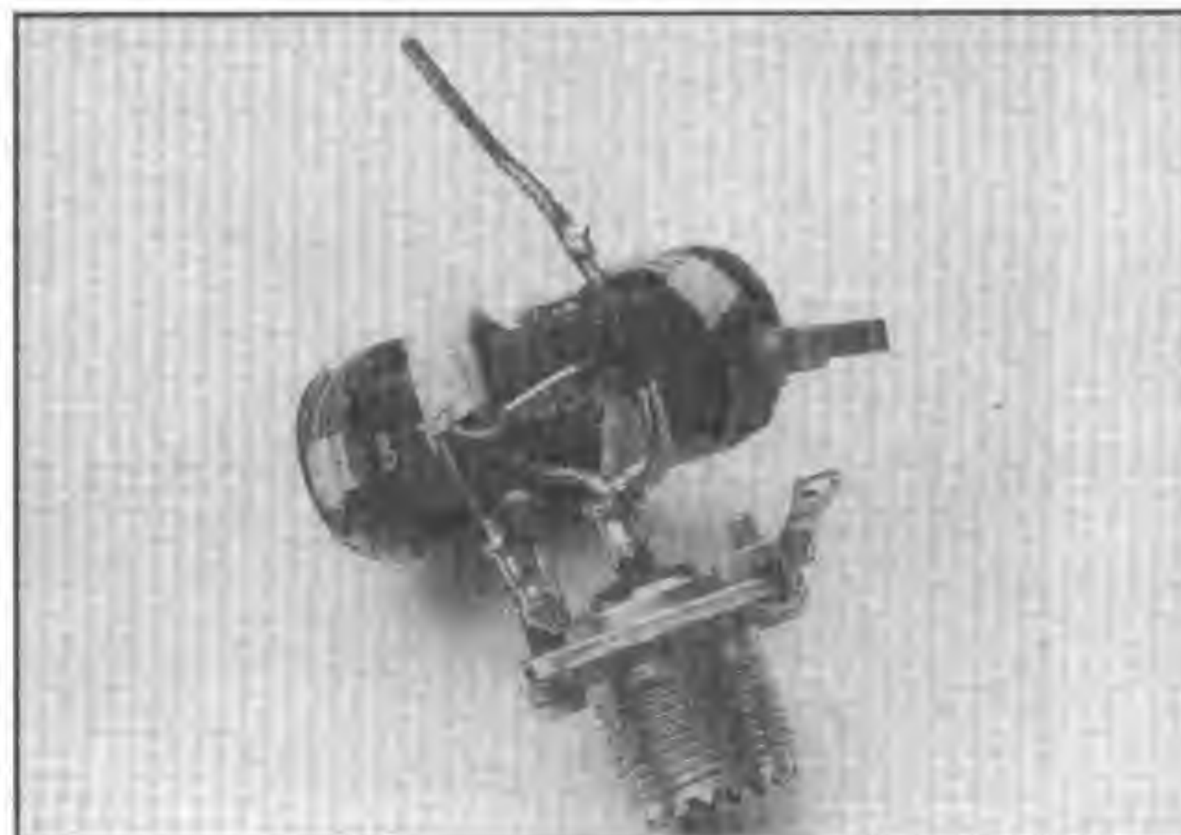
Figure 2 - Bottom-view of the highly efficient and broadband W2FMI-2:1-HDU100 transformer.
