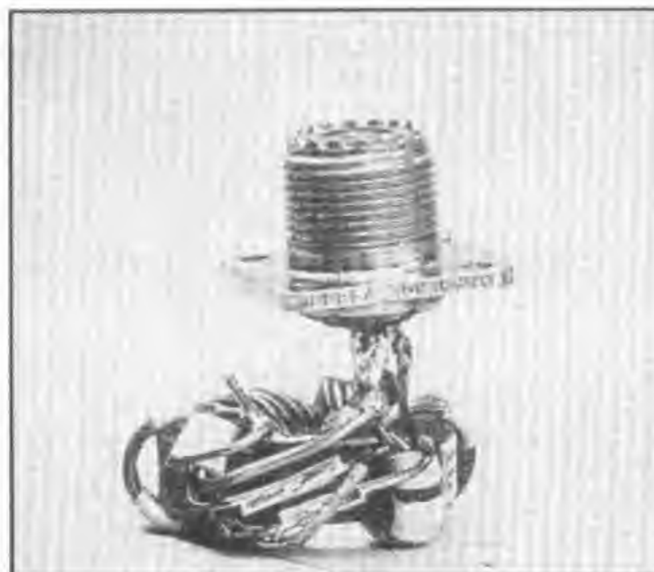
Figure 2 - Bottom-view of the highly efficient and broadband W2FMI-1.56:1-LDU50 transformer.
