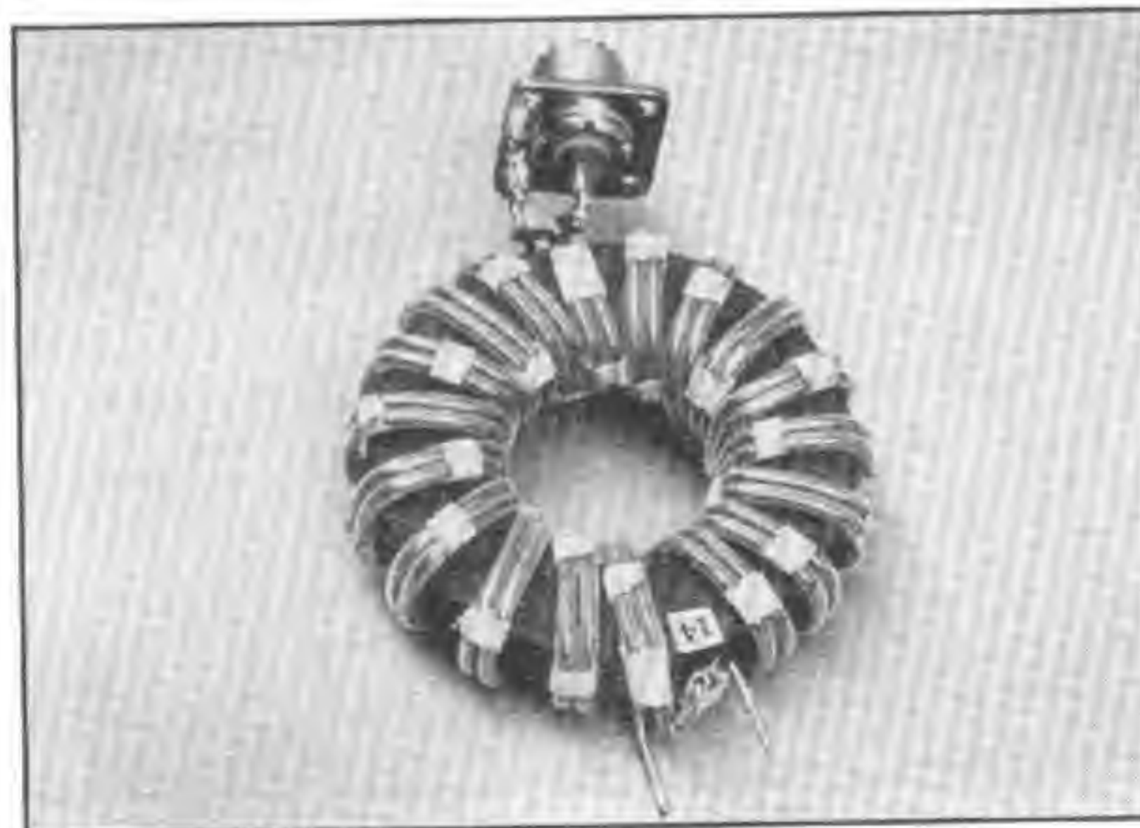
Figure 2 - Bottom-view of the very rugged, high power W2FMI-4:1-HBH200 transformer.
