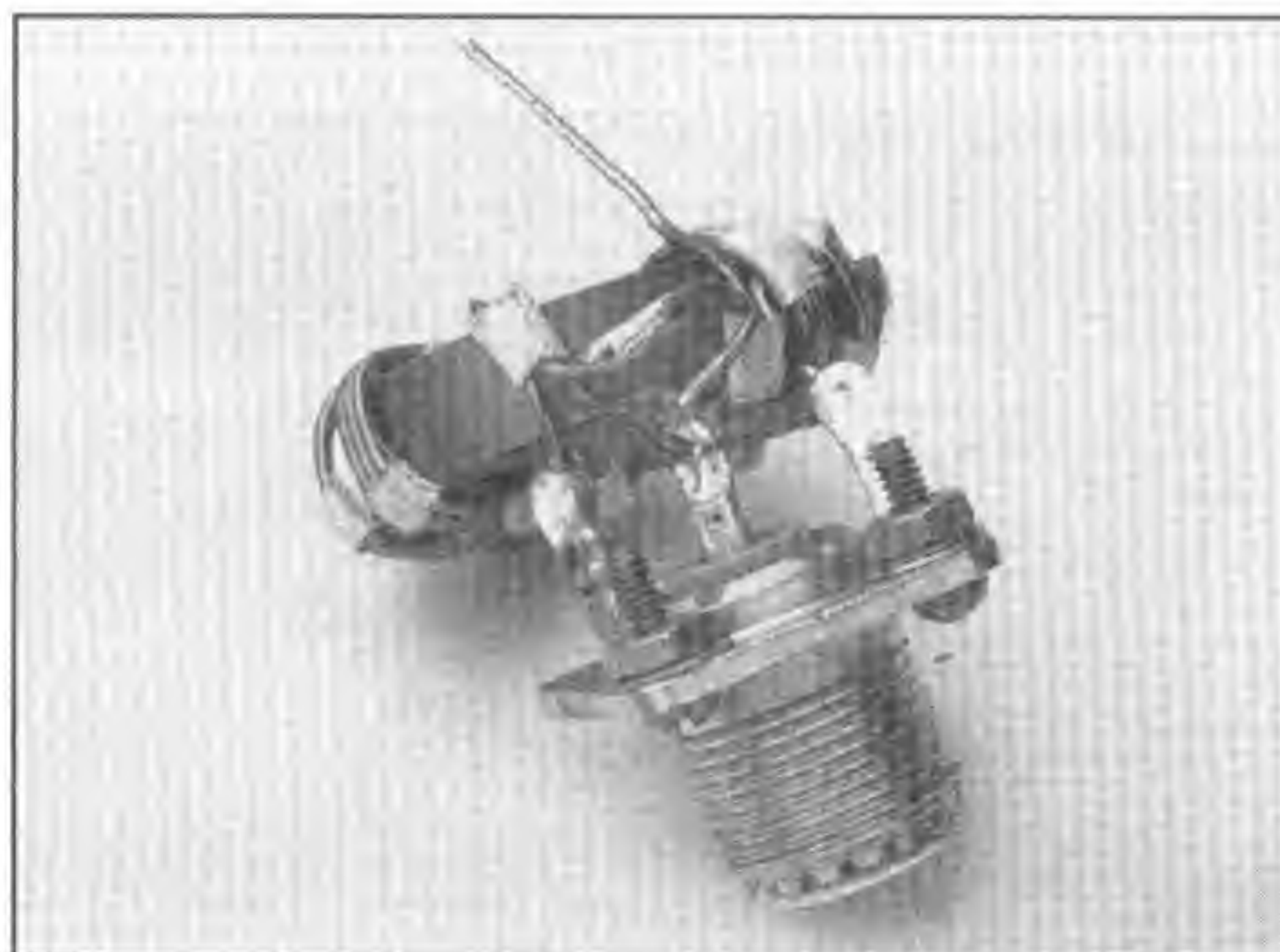
Figure 2 - Bottom-view of the highly efficient and broadband W2FMI-2.25:1-LU112.5 transformer.
