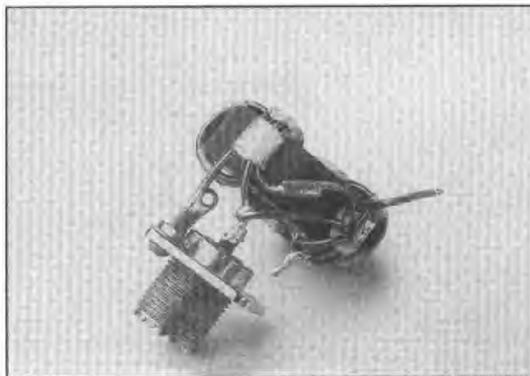
Figure 2 - Bottom-view of the highly efficient and broadband W2FMI-1.78:1-HU50 transformer.
