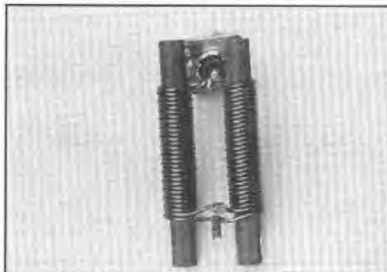
Figure 2 - Bottom-view of the high-power and broadband balun W2FMI-4:1-HB50 transformer.
