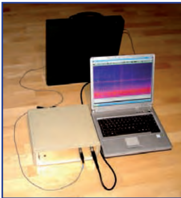
Figure 2. The receiver and power supply mounted in a small plastic housing. The connections go to the pick-up coil (in the black box) and to the laptop soundcard. The laptop is running CoolEdit.
