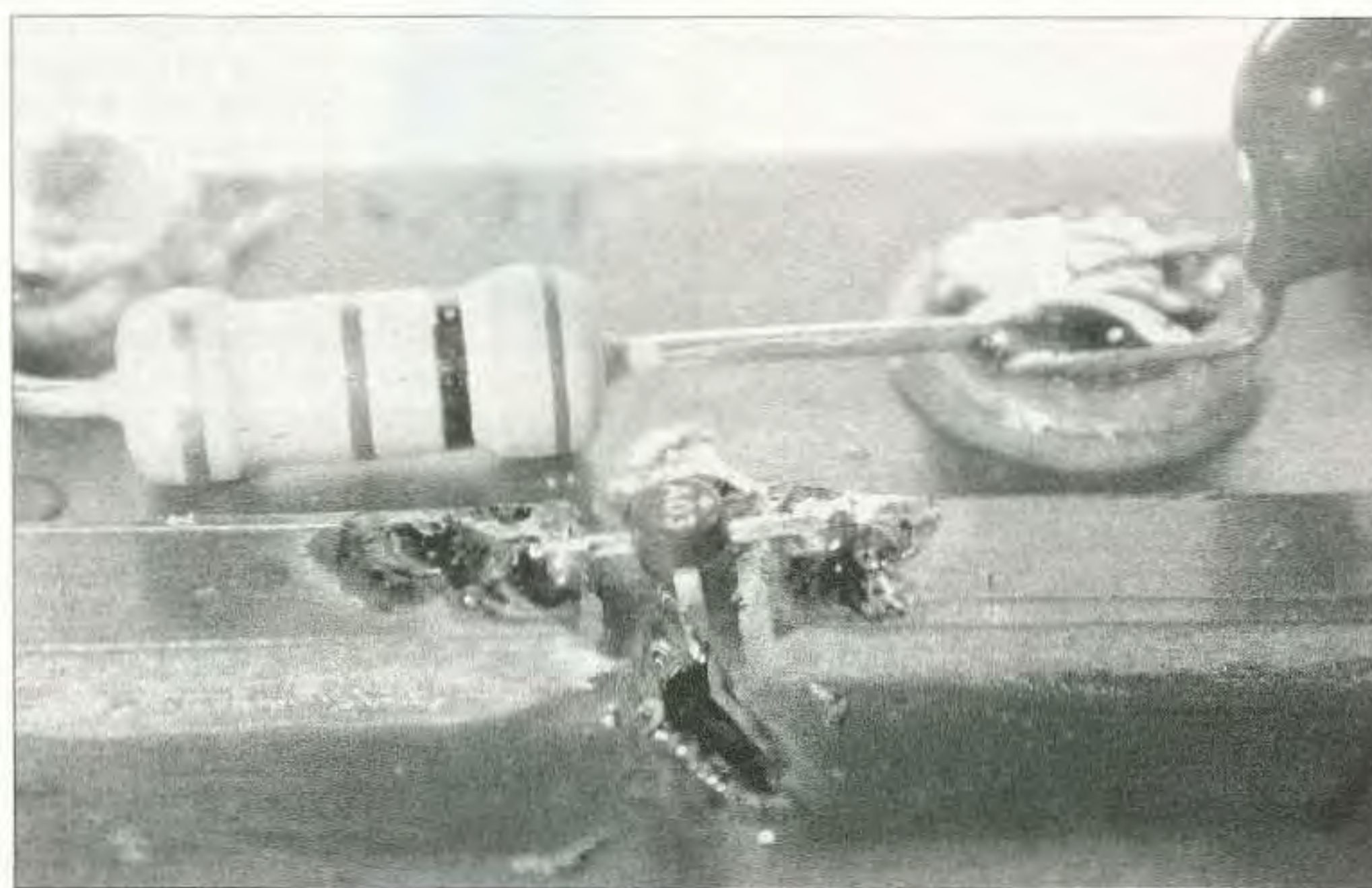
Photo G. MAR-3 amplifier in the test fixture, showing Manhattan construction, including strip lines.
