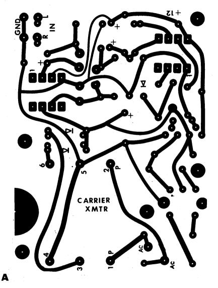
Fig. 5. Etching and drilling guide for the transmitter are shown above (A). Component placement for standard transmitter is at left (B). If pre-emphasis is used, the component placement at right is necessary (c).
