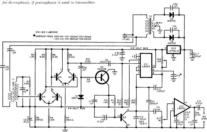
Fig. 3. In the receiver, the value of C10 must be increased
