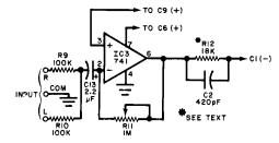
POPULAR ELECTRONICS' performance tests verified that the SIN ratio measured -65 dB, exceeding the author's claimed -50 dB. With "A" weighting it was -93 dB. At 0.9 W. distortion was 0.98%; at 2.5 W, it was 4.9%. Frequency response was 30 to 17,000 Hz ±0.5 dB-Ed.
