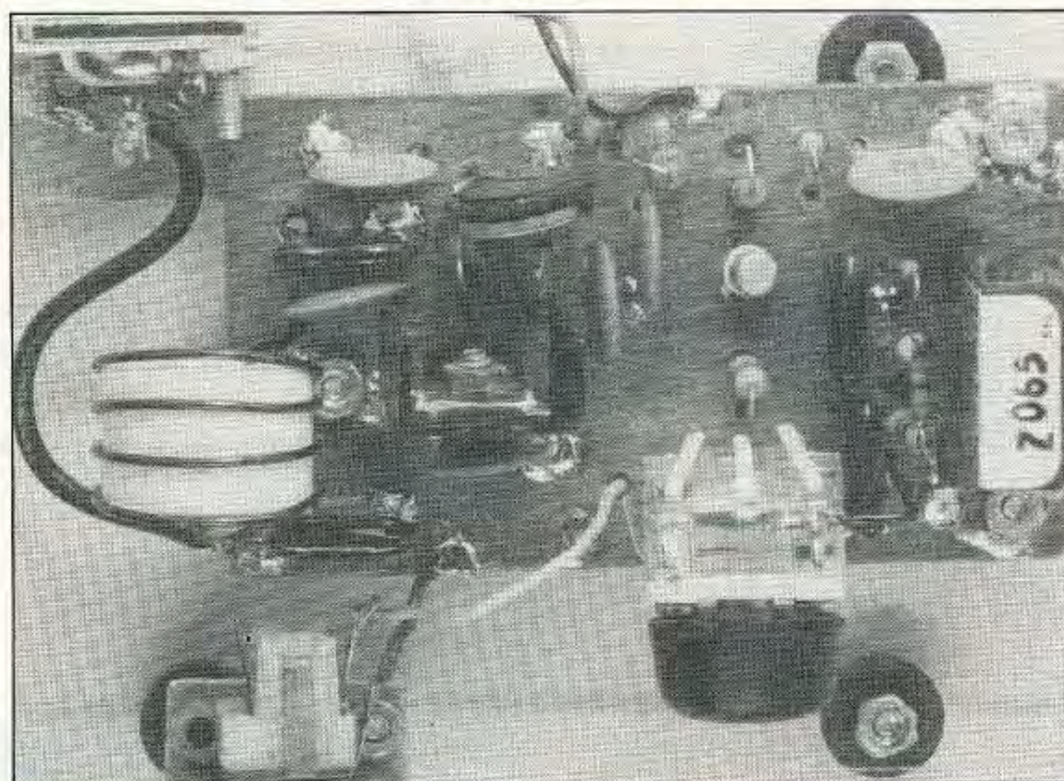
Photo B. Rock Bender au naturel. The board is mounted on a clear piece of Plexiglas™. The PL-259 antenna connector is wired to the board via RG-158 miniature coax. A key jack is at lower left.
