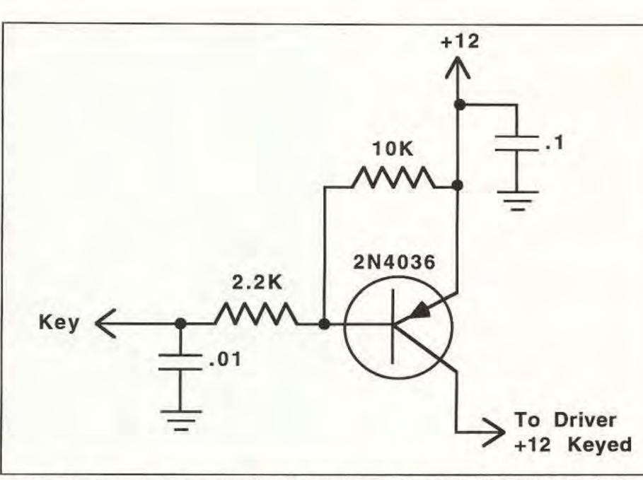
Figure 2. Schematic for an optional keying transistor and how you would interface it to the project.
