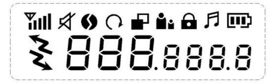
**1) RSSI** (Receiving Signal Strength Indicator) or TX Bar Icon Indicates the receiving signal strength during transmission and it can be indicated the number of bar according to the strength of receiving signal. It (TX Bar) is not transformed.
