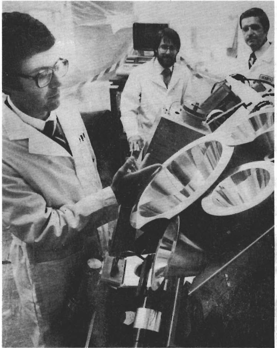
Part of the SEEP experiment carried aboard the S 81-1 satellite. Circular objects in the foreground are thermal radiators, used as part of the cooling system for the electron sensors which must operate at low temperatures for best sensitivities.
