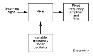
**Figure 3** The basic idea of a superhet receiver
