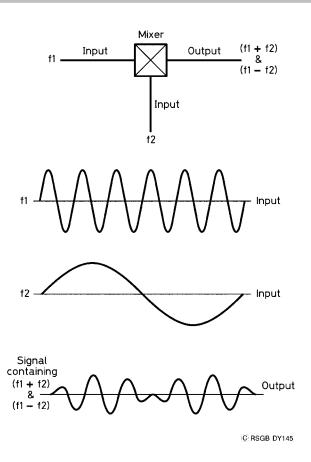
**Figure 1** The effect of multiplying (or mixing) two signals together
