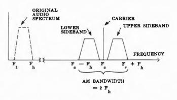
Figure 4 FREQUENCY SPECTRUM SHOWING AM BANDWIDTH REQUIRED TO TRANSMIT A TYPICAL AUDIO SPECTRUM
