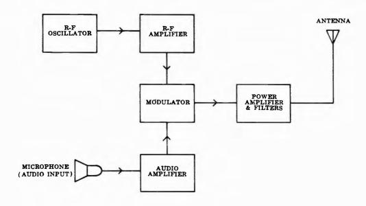
Figure 5 STANDARD BROADCAST TRANSMITTER
