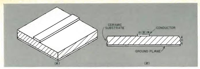
Fig. 1. Thin films of a flat, rectangular conductor strip deposited on side of a ceramic substrate with a conductive ground plane on the other side make up the microstripline circuit.
