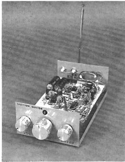
FIG. 2—THE COMPLETED MONITOR. The telescoping antenna is connected to J5 via a BNC-to-“F”-type adapter.
