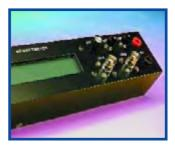
The button simply does not what it's supposed to do. In the mean time I managed to find the solution. In the hex file on your website (and that of the author, OZ2CPU), address 2007h (configuration word) reads 3375h. Consequently bit 11 is set, causing the background debugger to be enabled. However, pin 27 (Menu button), is then erroneously assigned to debugging instead of controlling the menu.
