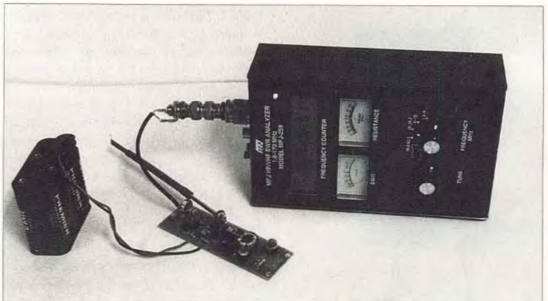
Photo D. Setting the output impedance.
