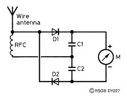
Figure 2 Field strength meter
