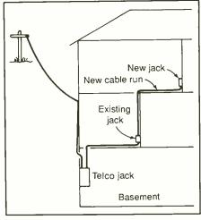
Fig. 10. A typical residential telephone wiring scheme.
