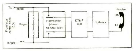
Fig. 6. Simplified diagram of a conventional single-line telephone.
