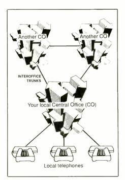
Fig. 7. All local phones connect to a Central Office, which is responsible for interconnecting instruments within its exchange area and connecting its local phones to other Central Offices for out-of-area calls.
