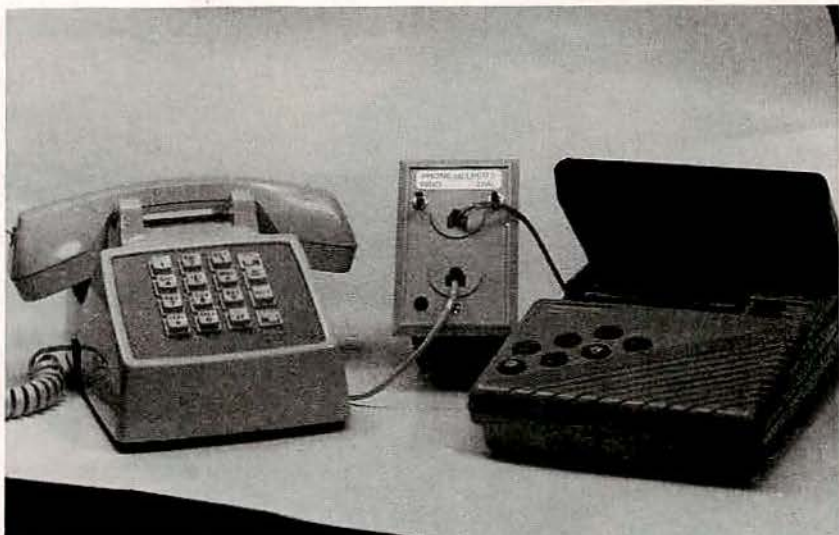
FIG. 5—SETUP FOR TESTING AN ANSWERING MACHINE with phone helper.
