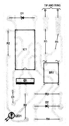
FIG. 2—IF YOU'RE USING A PC board, follow this parts-placement diagram. The LED can be mounted so that it can be bent in any direction, or remain straight up.
