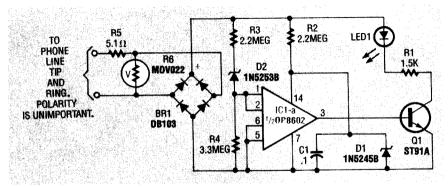
FIG. 1—AT THE HEART of the circuit is an ultra-low-current voltage-level sensor that draws only about 5  $\mu\text{A}$  when the phone line is not in use.
