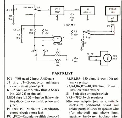
Complete schematic diagram of the automatic telephone disconnector circuit.
