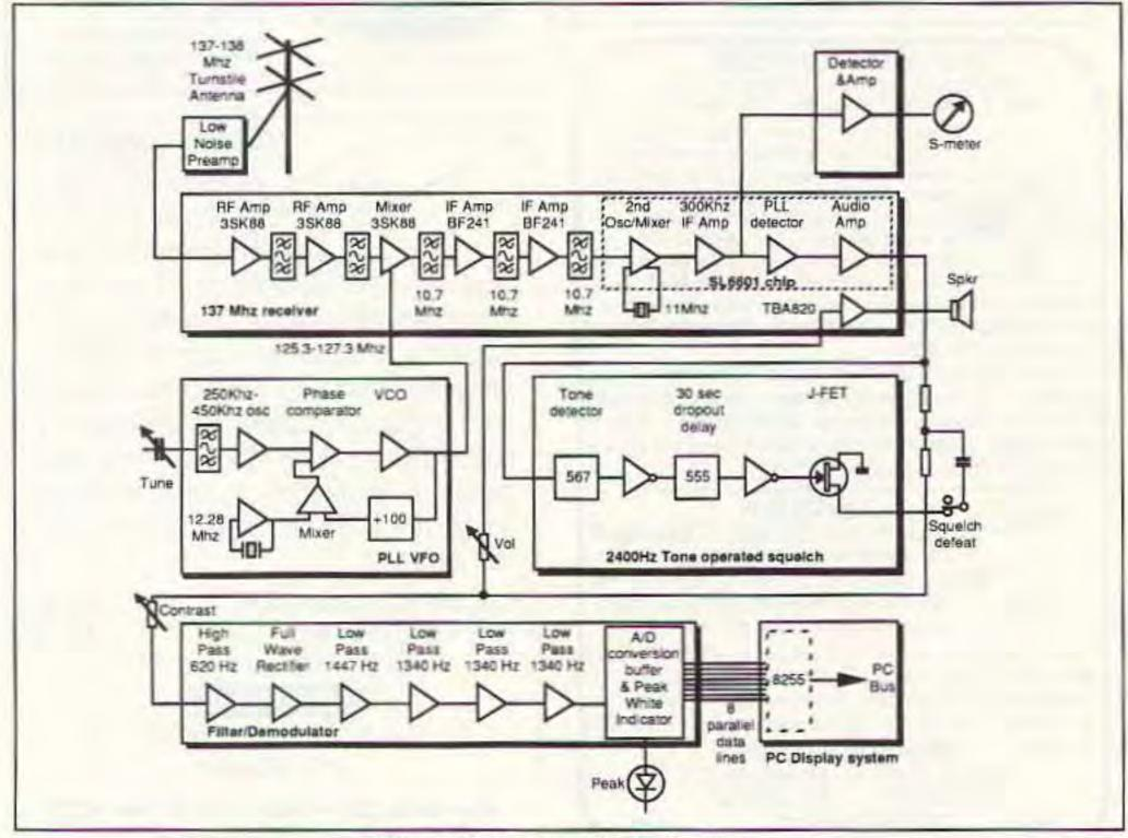
Figure 5. Station block diagram.
