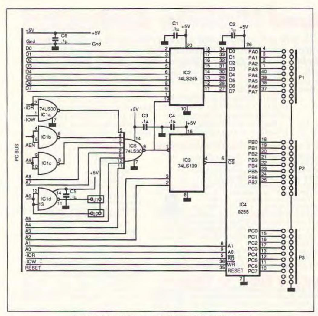
Figure 1. Circuit diagram of the parallel interface card.
