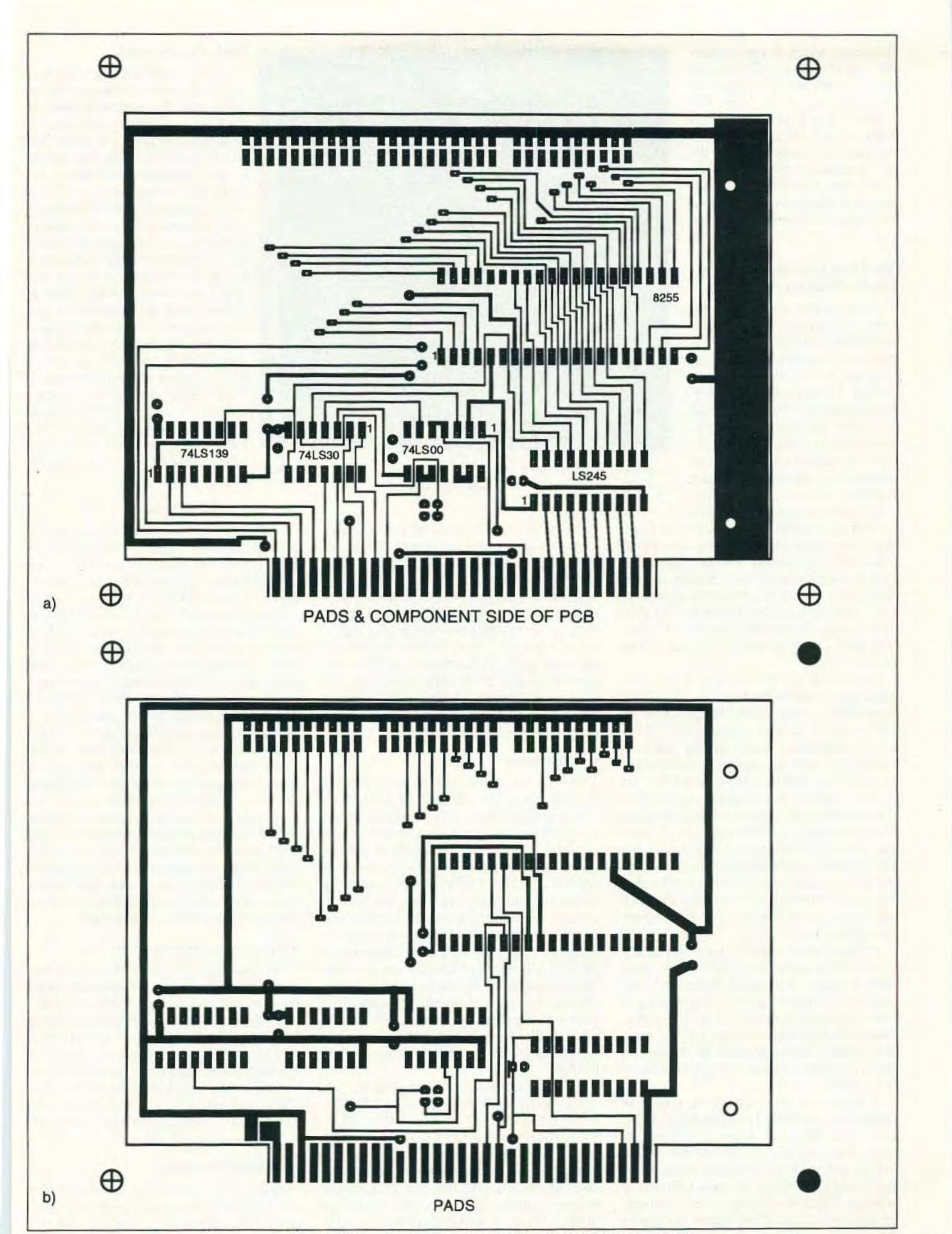
Figure 3a.) 1:1 PCB layout, component side; b) 1:1 PCB layout, solder side.
