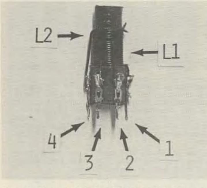
Photo A. Close-up of the L1-L2 inductor. L1 is 12 ccw turns and L2 is 4 ccw turns of #24 enameled wire. L3 is 35 cw turns of #32 enameled wire. All inductors are wound on a 1/4-inch slug-tuned coil form.
