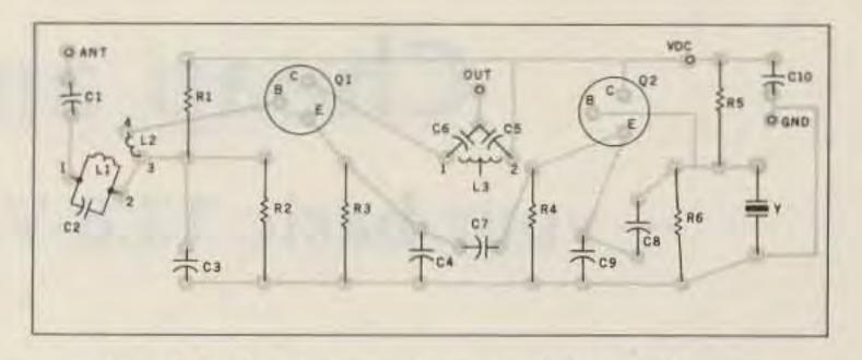
Fig. 3. Parts placement guide (foil side shown).
