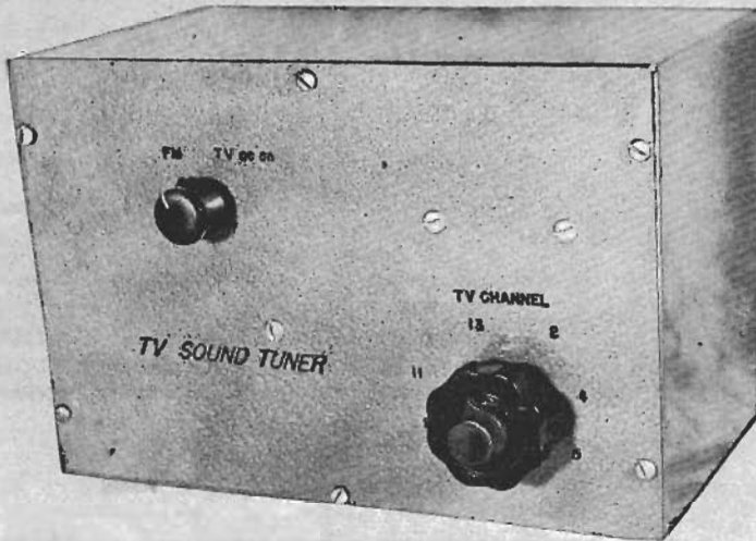
Panel view of tuner. In FM position, switch provides feedthrough to FM tuner from antenna input.
