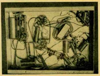
Under-chassis wiring is not critical except for the filament leads.
