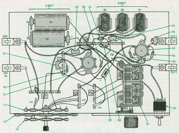
Fig. 8. Here is an overhead view of the finished receiver, showing the locations of the nonbaseboard mounted components. Follow closely the instructions in the text while referring to this diagram and Fig. 2 for guidance.
