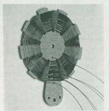
The rear surface of L2 should look something like this before it is mounted to the frame of the radio. Remember that the taps after turns 48 and 66 consist of two wires each, one coming from and one going to the coil form. The start wire extends up from the small hole on the left. The finish wire is pushed through the small hole on the right after turn 74.
