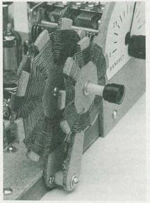
Here's how L2 and L3 are mounted to the front of the radio. Regeneration is controlled by moving L3 (the tickler coil) back and forth in front of L2. Note the short plastic spacer between the two coil forms near the bottom of the coil assembly.
