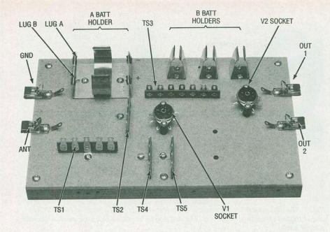
Fig. 2. Once the terminal strips, Fahnestock clips, battery holders, and vacuum-tube sockets have been mounted, the baseboard of your radio should look something like this. Refer to this illustration for the general layout of the baseboard and the locations of the terminal strips to which the interconnecting wires and components are connected.
