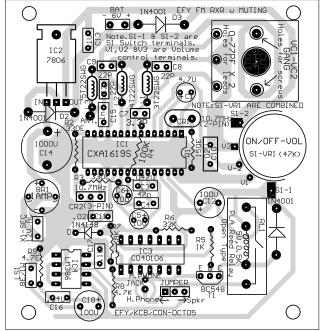
Fig. 5: Component layout for the PCB
