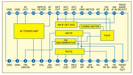
Fig. 1: Functional block diagram of Sony CXA1619S
