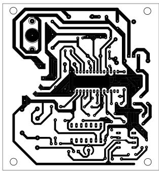
Fig. 4: Actual-size, single-side PCB of noise-muting FM receiver
