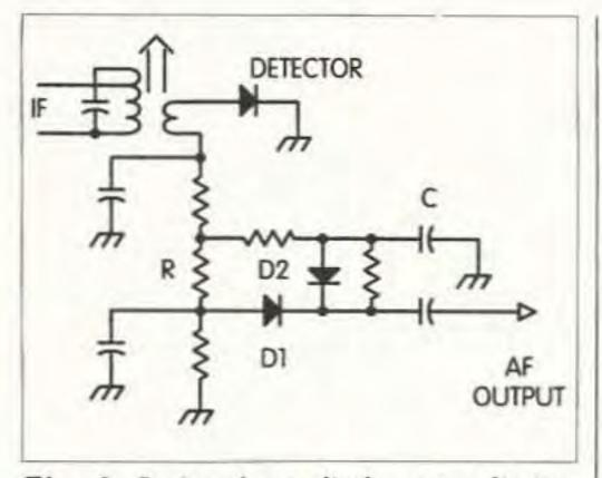
Fig. 6. Series-shunt diode noise limiter used with an AM detector. Capacitor C establishes a long time constant to hold the switch threshold during a noise pulse.
