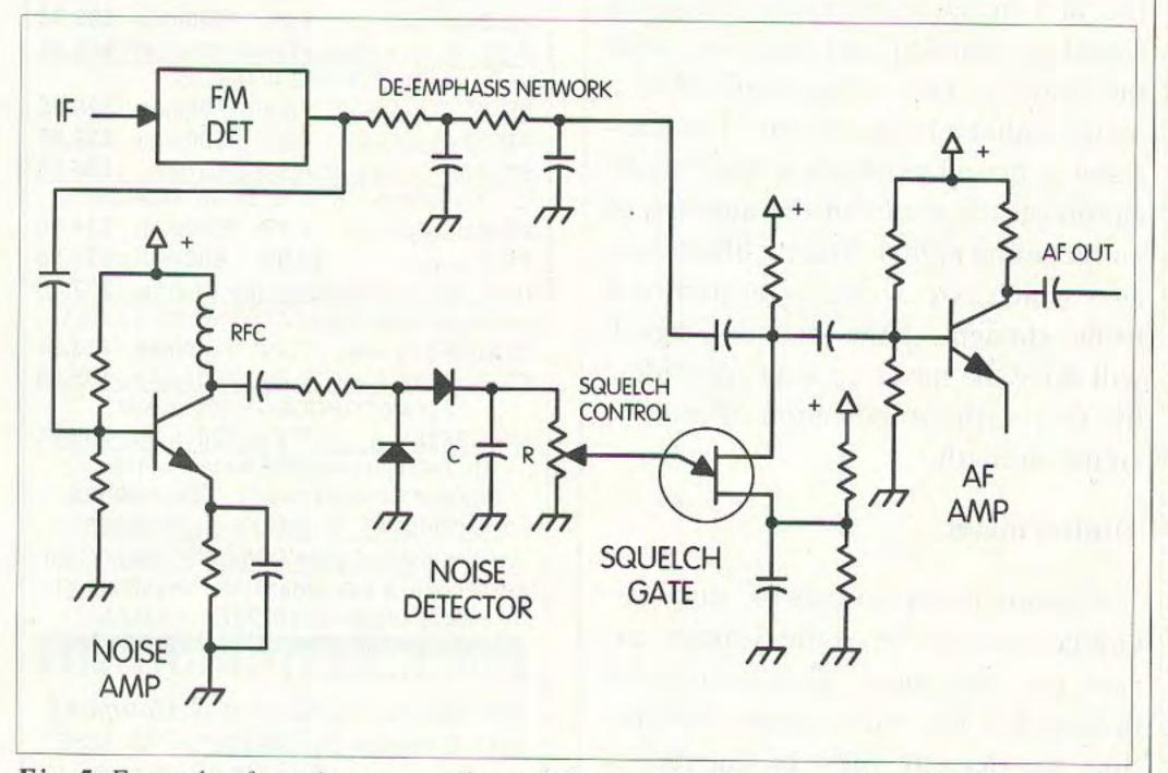
**Fig. 5.** Example of a noise-operated squelch gate. The function is based on the presence of white noise in the signal channel during the absence of an incoming signal. Values of C and R establish a time constant for opening and closing the squelch gate.
