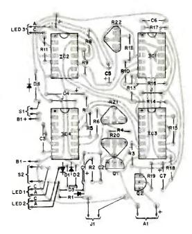
er than soldering them directly to the board. This makes replacement of defective ICs infinitely easier and eliminates the possibility of damaging them during soldering. Be sure to observe polarities and pin basings when you mount the diodes, transistors, LEDs, ICs, and electrolytic capacitors.
