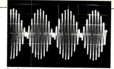
Fig. 1. Oscilloscope photo of the alert signal of the Emergency Broadcast System. It consists of two tones at 853 Hz and 960 Hz broadcast for 22.5 seconds.
