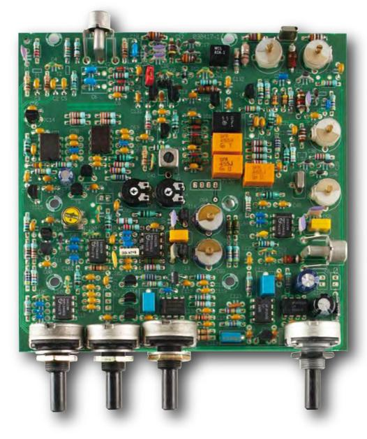
large input signals. Eagle-eyed readers will have noticed that we've swapped the input (RF) and output (IF) of this mixer. The mixer still works well in this configuration, but it has the advantage that the input frequency can be a lot lower (almost down to 0 Hz, which is exactly what we require).
