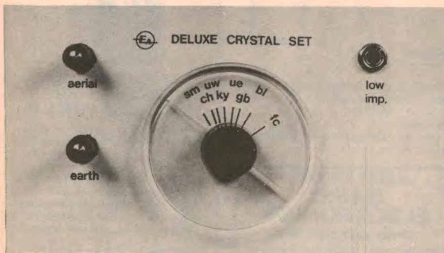
Front panel of the deluxe crystal set. Note the simple handspan dial with the station markings behind it. The panel was made from stiff card, using Letraset rub-on letters.
