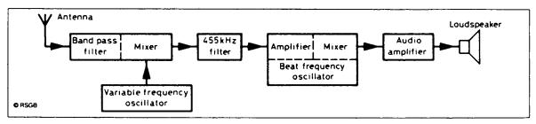
Figure 1 This is how the different stages of the Colt go together to make a superhet receiver
